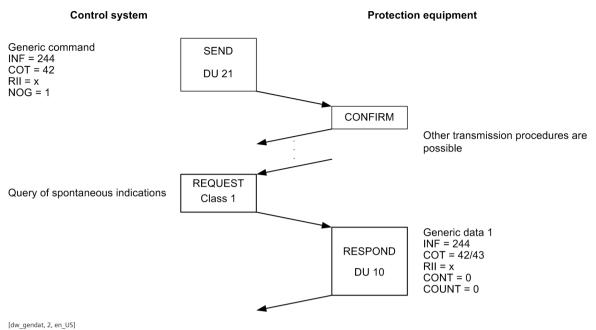
Figure 6-6 Reading an Individual Parameter
