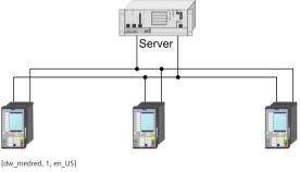
Figure 6-3 Media Redundancy
