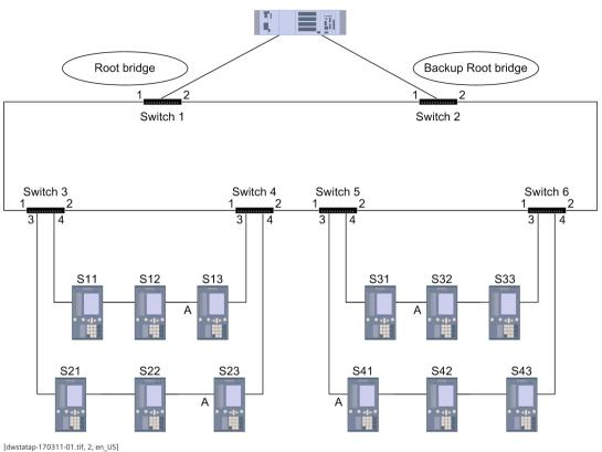
Figure 1-13 Structure with Alternate Ports
