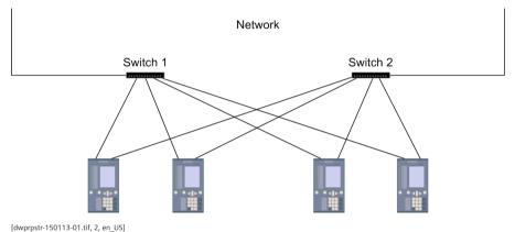
Figure 1-11 SIPROTEC Devices Connected via 2 Independent Networks (LAN A and LAN B)
