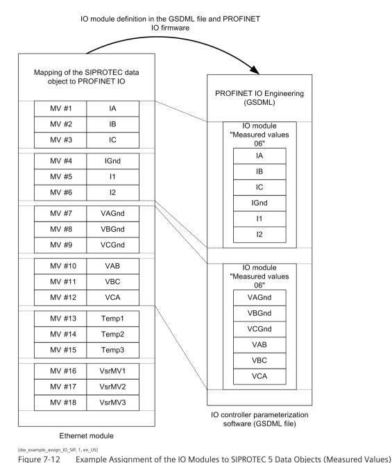
For example, if the SIPROTEC 5 device provides 18 measured values (MV#1 to MV#18). However, only 12 measured values (current, voltage) can be transmitted and assigned to the PROFINET IO mapping in DIGSI 5 (MV#1 to MV#12). In this case, you have 2 choices as follows:
