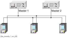
Figure 6-4 Master Redundancy
