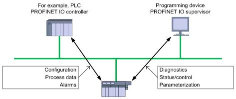
Field devices PROFINET IO device
