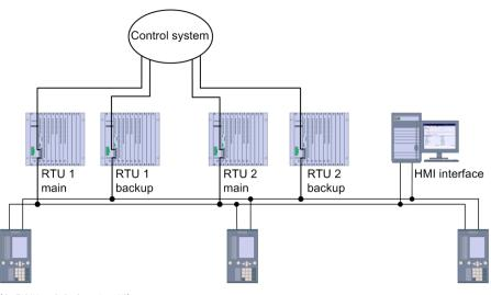
[dw\_T104MasterRedundancy, 1, en\_US] Figure 4-4 Master Redundancy
