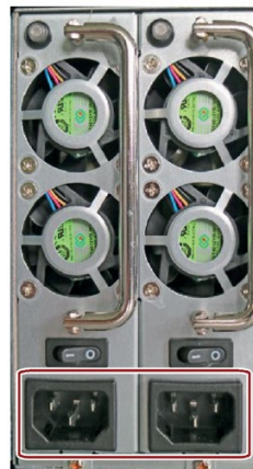
Redundant power supply
