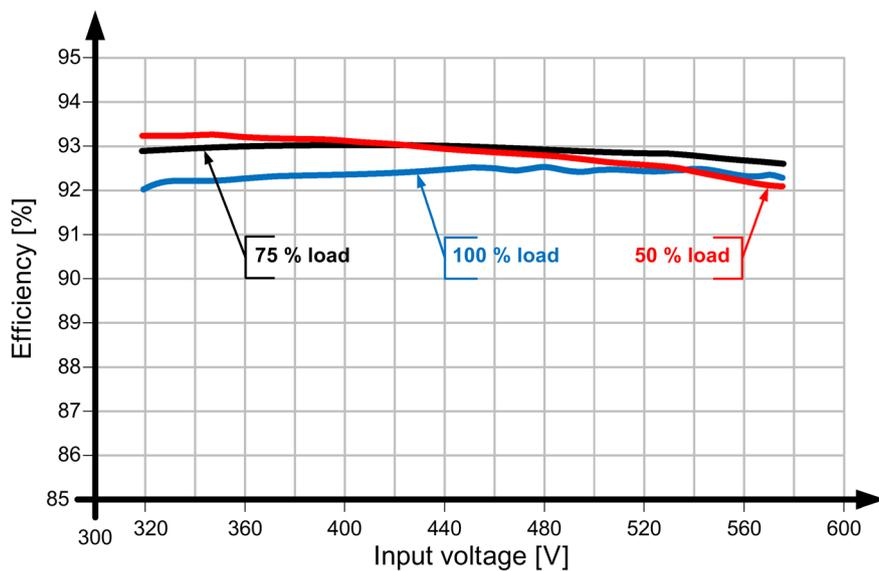
Figure 6-10 Efficiency 6EP1437-3BA10
