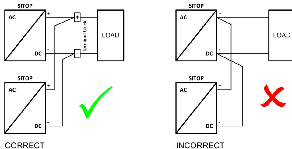
Figure 9-1 Parallel connection
