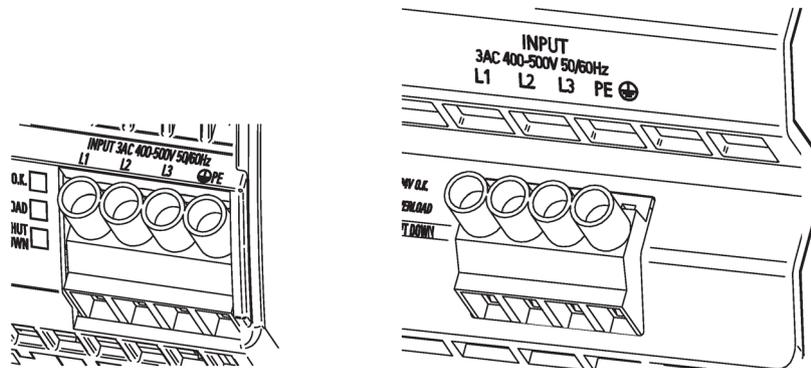
Figure 5-1 Line supply connection
