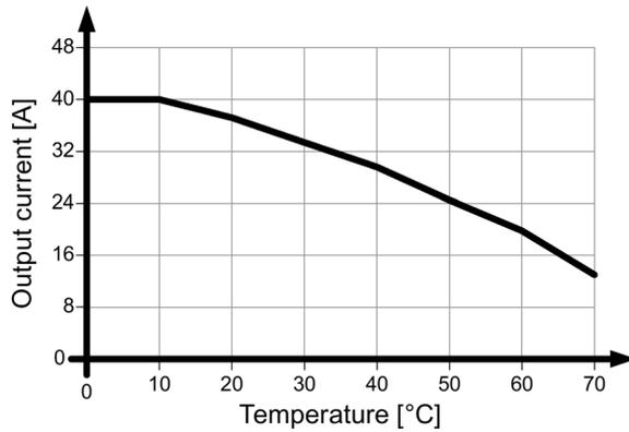
Figure 4-9 6EP1437-3BA10 mounting position (1)
