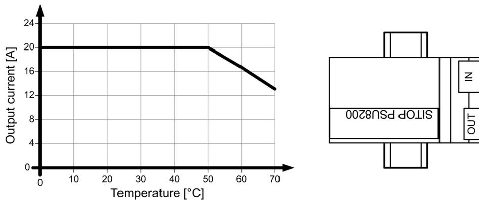
Figure 4-4 6EP3436-8SB00-0AY0 mounting position (1)
