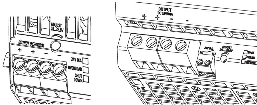
Figure 5-2 Output connection
