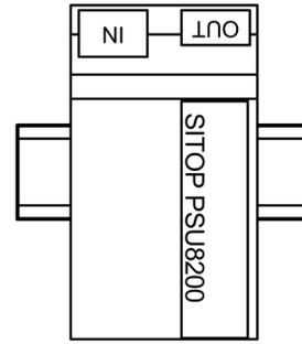
Figure 4-6 6EP3436-8SB00-0AY0 mounting position (3)
