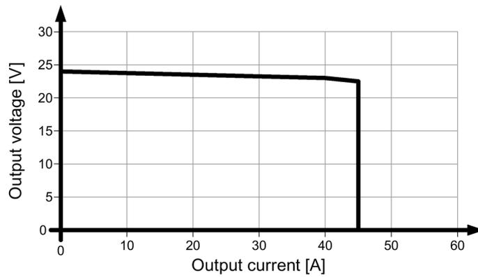
Figure 6-6 6EP1437-3BA10 parallel operation output characteristic curve
