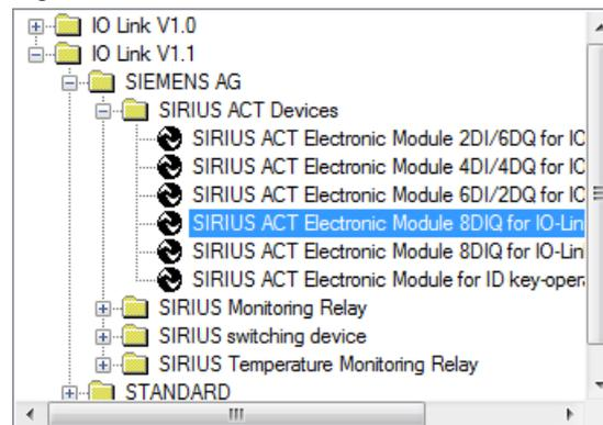
5. Select "SIRIUS ACT electronics module for ID key switches" from the catalog under "IO Link v1.1 > SIEMENS AG > SIRIUS ACT devices" and move it to port 2 in the normal working range.
