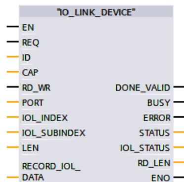
Data set 94 contains the ID of the inserted ID key. The record is requested from the electronics module with a positive edge at the "REQ" input. The trigger used is the "ID key detected" signal from the process image of the inputs.
