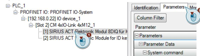
7. If necessary, adapt the settings of the inputs/outputs. The default setting of 6 inputs and 2 outputs is suitable for this application example.
