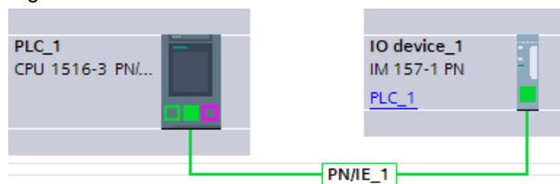
7. Double-click on the interface module to switch the device view.
