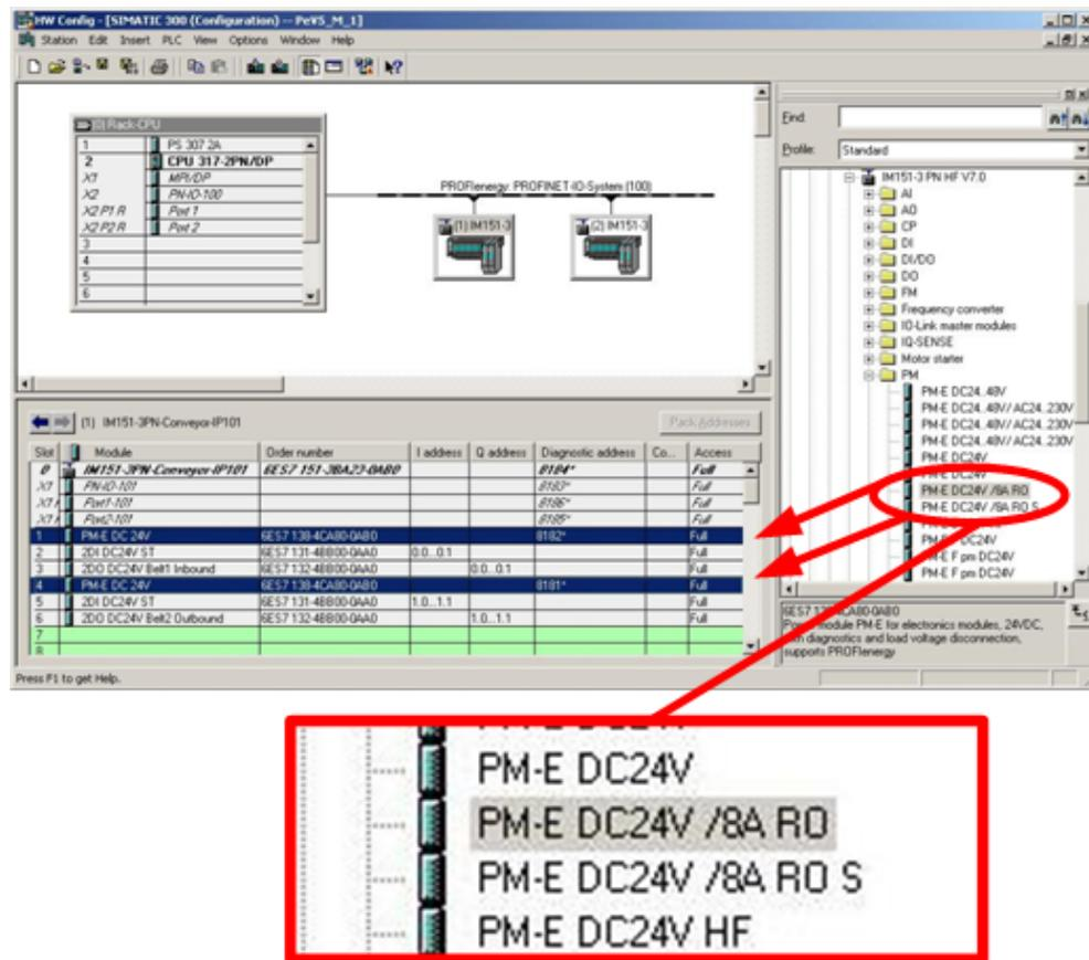
Equip the ET 200 S with at least one PROFEnergy-enabled power module. You are free to select the further equipment. You can either select further PROFEnergy power modules or any other modules.
