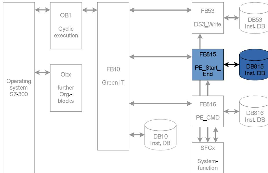
With the FB815 "PE\_START\_END" the pause is started or stopped for the determined PROFINET IO device, here ET 200S. The switchable blocks behave according to the settings of the FB53 "DS3\_WRITE". The parameter PAUSE\_TIME provides the switchable block with the planned pause time for control.
