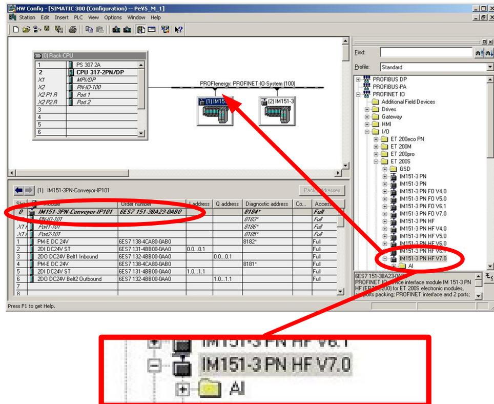
Select one of the PROFInergy-enabled head modules (V7.0) and add it to the PROFINet thread.
