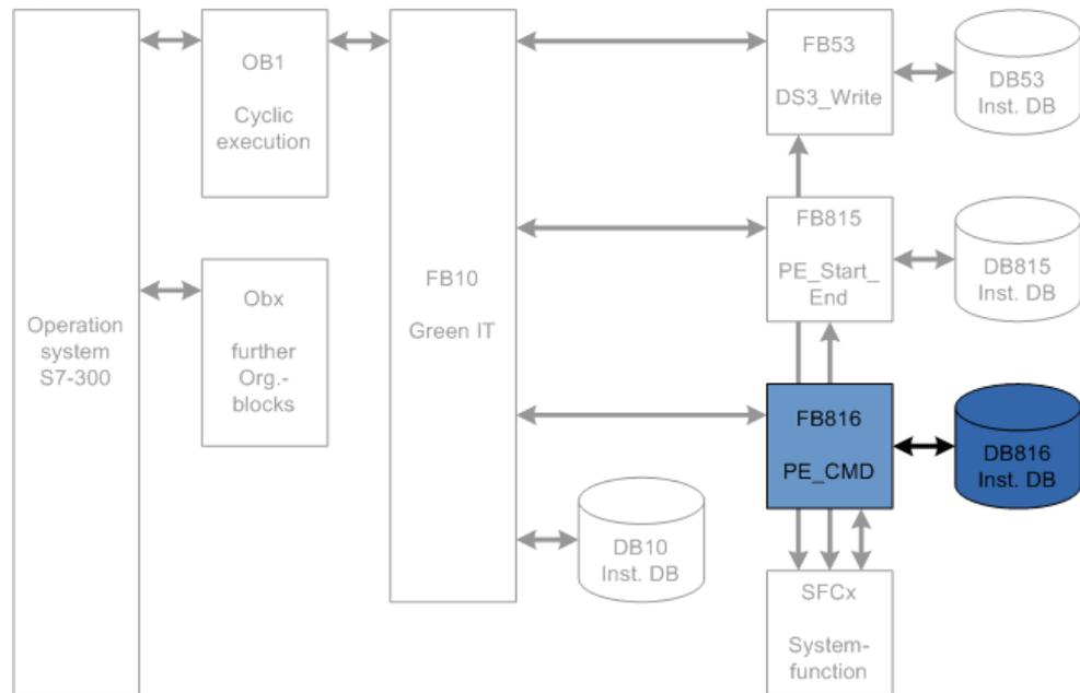
FB816 "PE\_CMD" is a transparent block to illustrate the complete PROFInergy standard. Due to its free parameter transfer the block is open for future extensions of the PROFInergy profile. To use this block advanced knowledge of the PROFInergy profile is required. That is why the reading of status information is shown exemplarily in this application.
