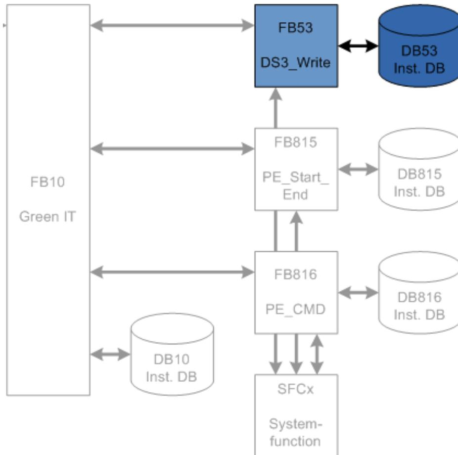
With the FB53 the switching behavior for up to 8 slots (here power modules) in a PROFINET IO device (here ET 200S) can be determined.
