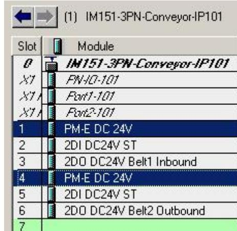
The screenshot shows a rack configuration window for a rack containing an IM151-3PN-Conveyor-IP101. The rack is divided into slots, with slots 1 and 4 highlighted in blue, indicating they are PROFlenergy-enabled power modules. The modules are listed as follows:
