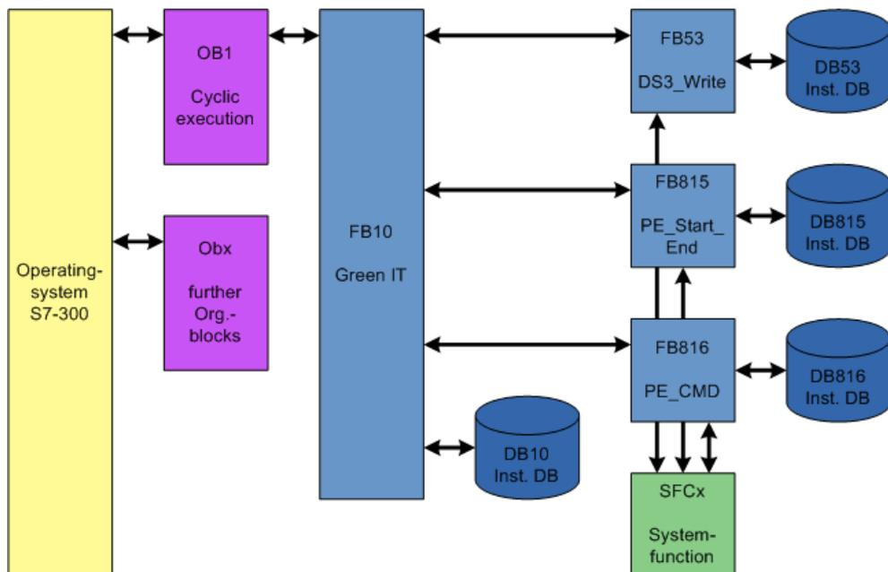
The function block FB 10 "GreenIT" bundles the actual PROFlenergy block calls and provides a comfortable interface for the HMI via its instance data block.
