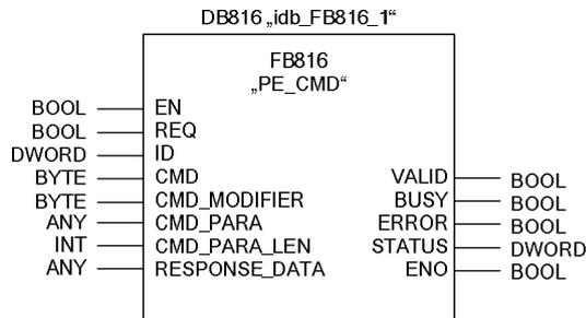
With this FB 816 PROFlenergy commands are transferred to a PROFlenergy-enabled device. The input data are stored in the data range "CMD\_PARA" which is addressed by the ANY-pointer. The output data are stored in the data range RESPONSE\_DATA which is addressed by the ANY-pointer.
