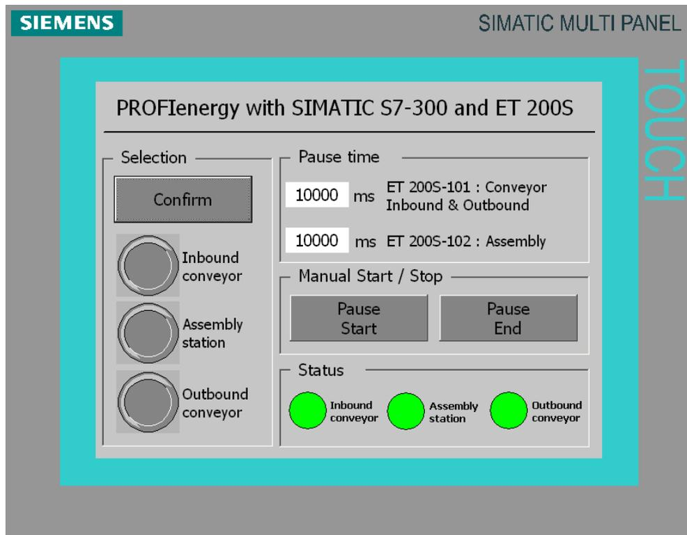
All used command bits refer directly to one or both instance data blocks (FB53 / FB815 for PROFInergy device 1 and 2).
