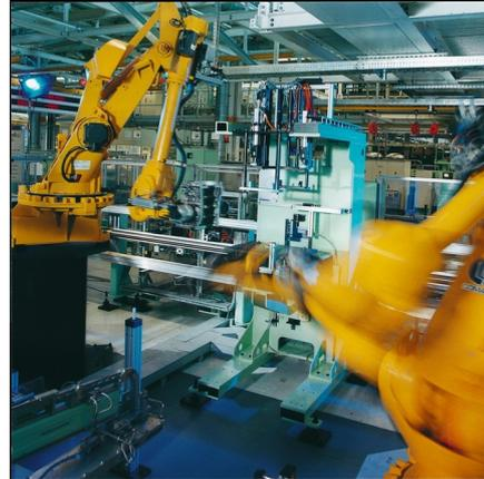
By using an example from the production – here a production line with robot – the switching off of the independent production unit (robot as i-device) is described in this application.
