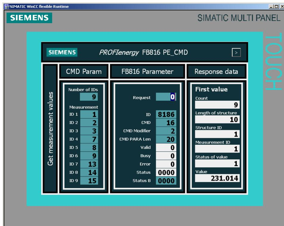
Changing the “Request” parameter from “0” to “1” triggers the read process. 9 IDs are read as listed in the left block. The first value is displayed in the right block.
