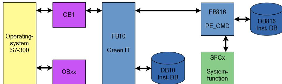
The function block FB 10 “GreenIT” bundles the actual PROFlenergy block calls and provides a comfortable interface for the HMI via its instance data block.
