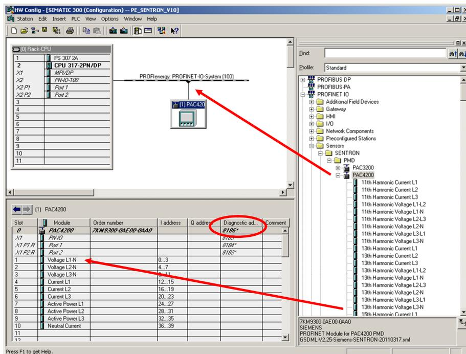
The project for this application already contains the GSDML for the SENTRON PAC4200 PROFINET communication module. If you are not using the project, install the latest hardware support package (HSP) or the GSDML for Sentron PAC PN module.
