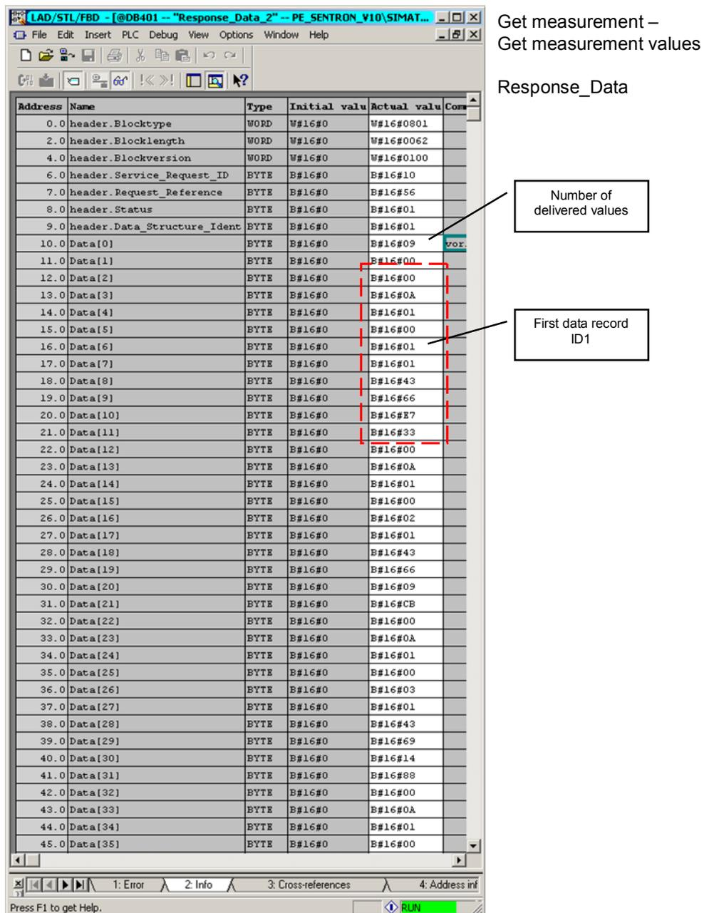
This figure shows the DB401 after the “Get measurement values” command. It contains the list supplied by SENTRON PAC with the requested measured values. If the DB is too short, a respective message is entered in *header.Status*.
