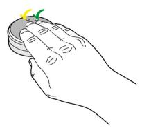
The contact remains closed while the hand remains in contact with the sensor switch surface. No force needs to be applied in order to actuate the switch.
