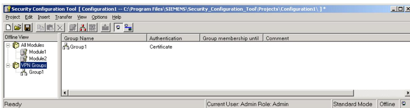
3. In the content area, select the SCALANCE S module "Module 1" and drag it onto "Group 1" in the navigation pane.
