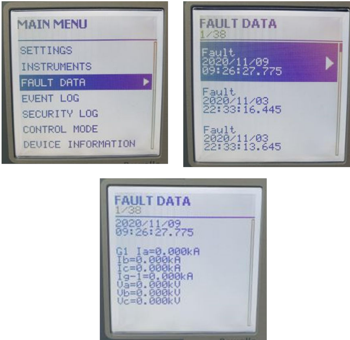
[sc_7SR5_DeviceFaultDataMenu, 1, --] Figure 7-8 Fault Data
