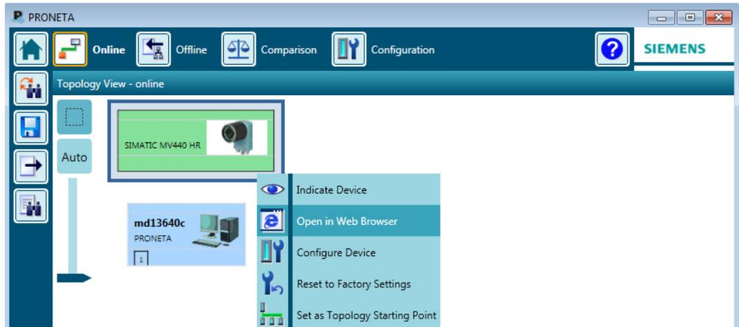
Figure 3-7 Network overview - opening the user interface of the reader
