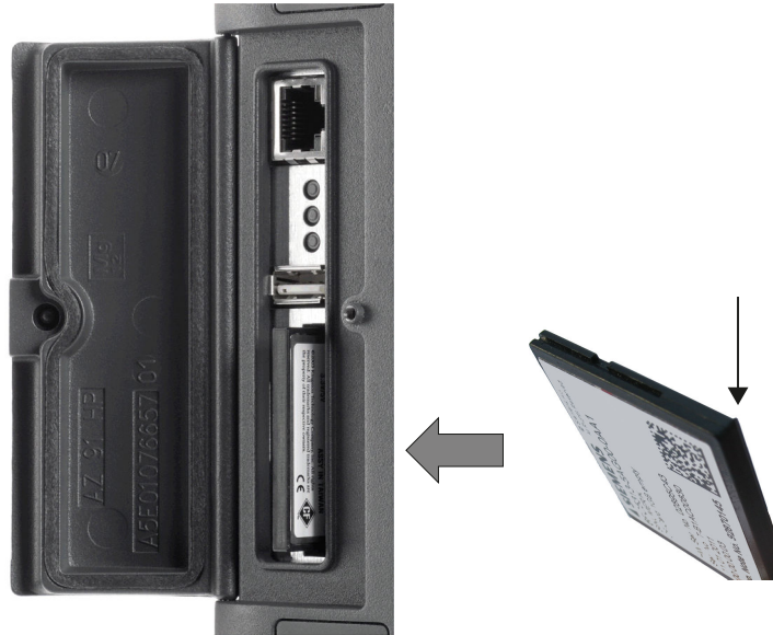
Figure 2-10 Direction to insert the user CompactFlash card
