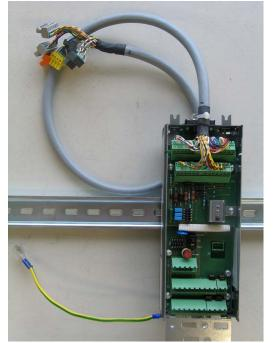
Figure 5-8 Connecting the long cable harness
