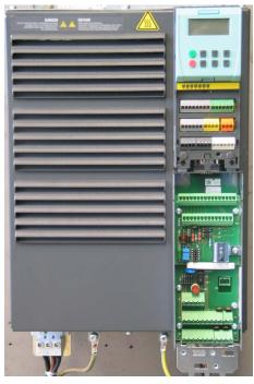
Figure 5-5 CM and CU without terminal cover
