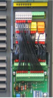
Figure 5-7 CM/CU wiring has been completed
