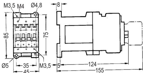
1) Minimum clearance from earthed parts 10 mm
