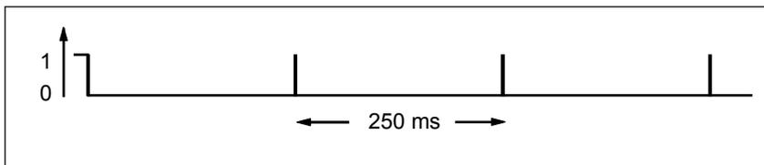
As soon as the time runs out, the timer is restarted. Because of this, the signal produces a signal state of 1 only briefly.
