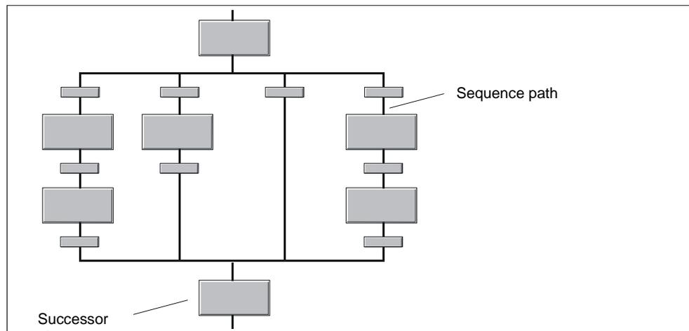
Fig. 1-9 : Example of an Alternative Sequence with Four Sequence Paths
