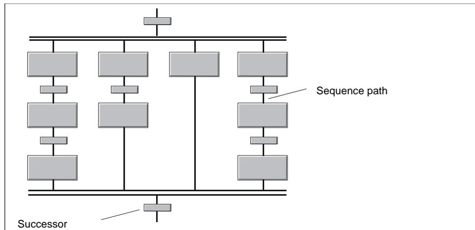
Fig. 1-8 : Example of a Simultaneous Sequence with Four Sequence Paths
