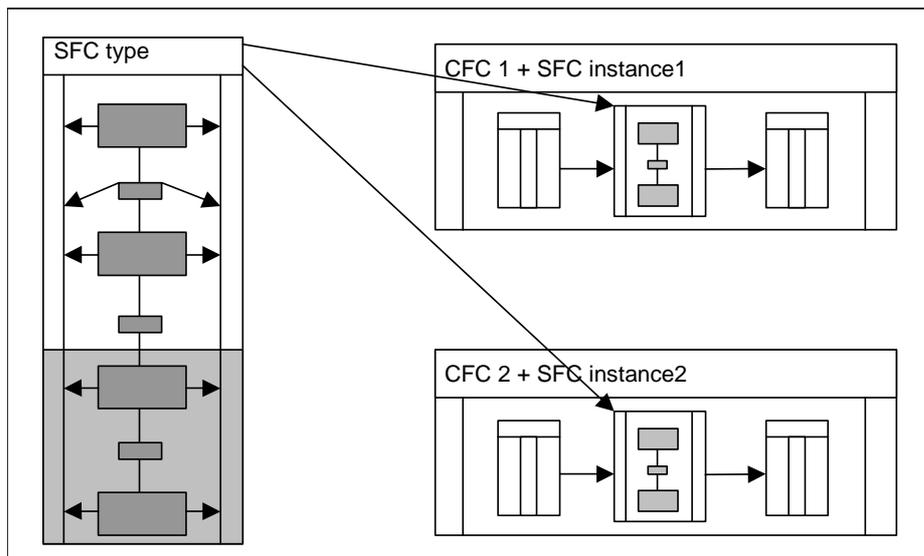
The properties of the SFC type and SFC instance include the name and comment as descriptive data and the SFC type also has the properties author, version and family and FB number as information for the compilation. Both for the SFC type and the SFC instance, you can specify the operating parameters for the CPU that determine how the instance executes on the CPU (for example mode, step control mode, execution options).
