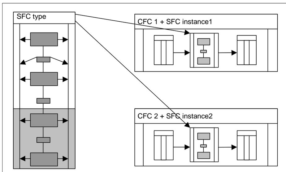
Fig. 1-2 : Interaction of SFC Type/Instance and CFC
