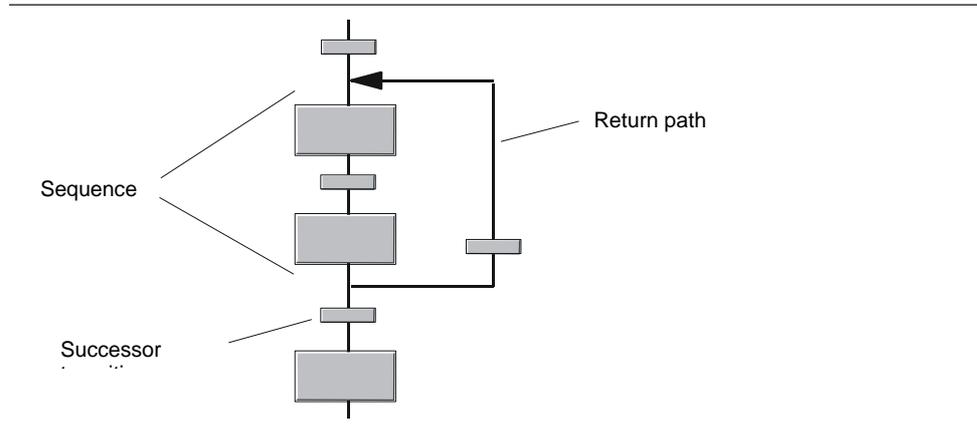
Fig. 1-10 : Example of a Loop
