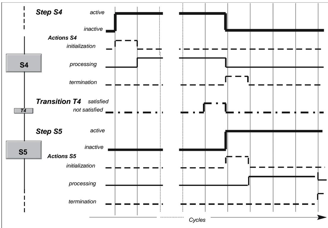
Fig. 3-4: Time Response in Executing Steps and Transitions in a Sequential Control System
