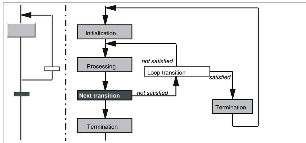
Fig. 3-5: Phases of a Loop
