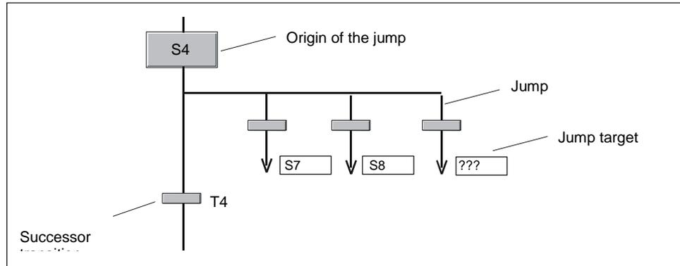
Fig. 1-11 : Example of the Origin of a Jump with Three Jumps
