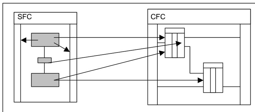
The properties of the SFC chart include name, author and comment as descriptive data and the operating parameters for the CPU that decide the execution (for example mode, step control mode, execution options).
