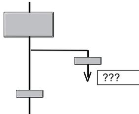
To insert a jump, click on the vertical link of the sequence immediately below a step. A simple click creates a jump with an undefined destination. The destination is displayed as question marks (???)
