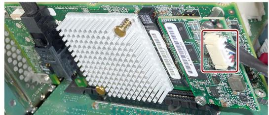
7. Insert the adapter cable at the marked position.
