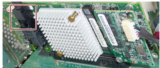
8. Connect the adapter cable to the required drives.
