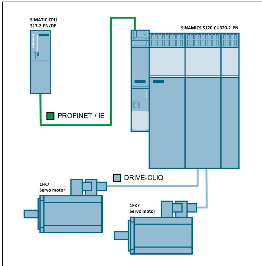
In this application description it is shown, how a SINAMICS S120 can be moved speed-controlled by means of a SIMATIC S7-300/400 (STEP 7 V5). For this purpose a communication via PROFINET IRT (isochronous) is configured between controller and drive.
