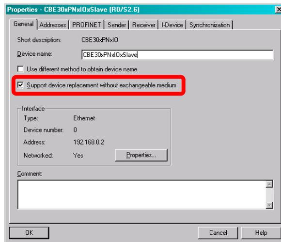
This properties window will open by double clicking on the PN interface of the IO-Controller in HW Config.
