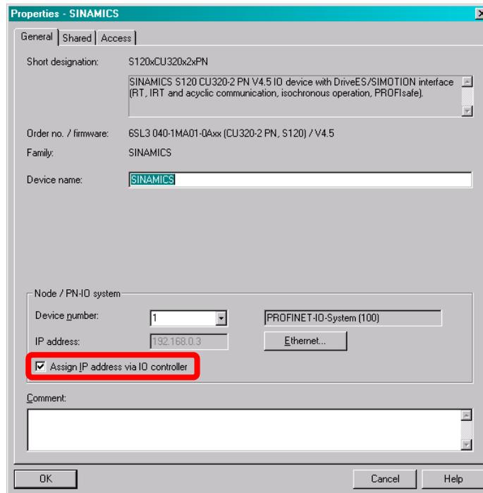
The received IP address from IO-Controller is just a temporary address (till next power OFF/ON of the device). The received address is higher prior as a fixed set IP address via engineering software.
