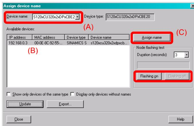
Select the configured device name (A) and select the corresponding device (B) and click on “Assign name” (C). The device name will be transferred to the device.
