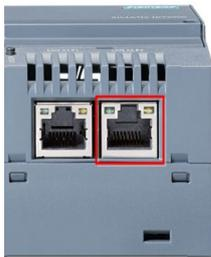
Figure 4-22 Connecting Ethernet Port X2P1 for data acquisition
