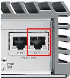
Figure 4-17 Connecting Ethernet Port X2P1 for data acquisition
