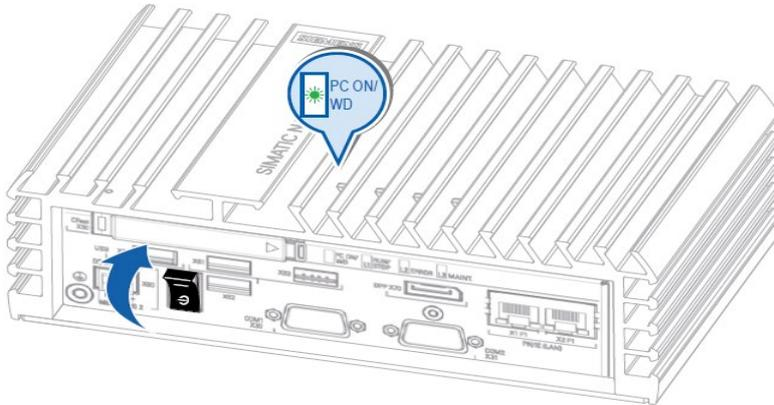
Figure 3-9 Set the switch to “ON” for MindConnect Nano
