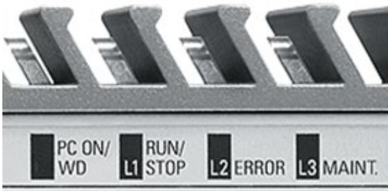
Figure 7-3 LED lights- bottom view 2
