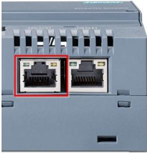
Figure 3-6 Connecting the port X1P1 for internet (MindSphere)
