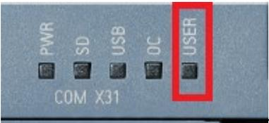
Figure 4-21 LEDs “PWR” and “User”
