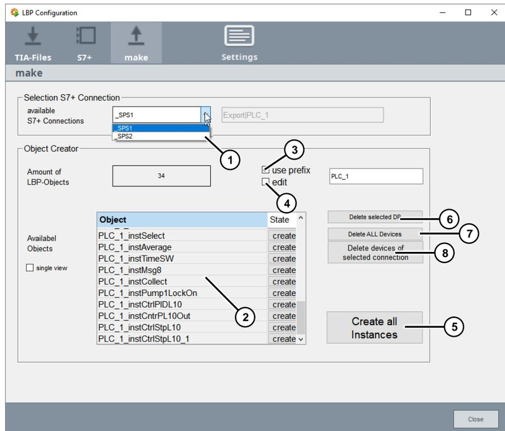
1. From the drop-down list in the “Selection S7+ Connection” (1), select the correct station from the control systems or configured connections. After selecting a connection, the LBP devices configured in the control system that are available for the visualization are automatically displayed and listed in the table at the bottom (2).
