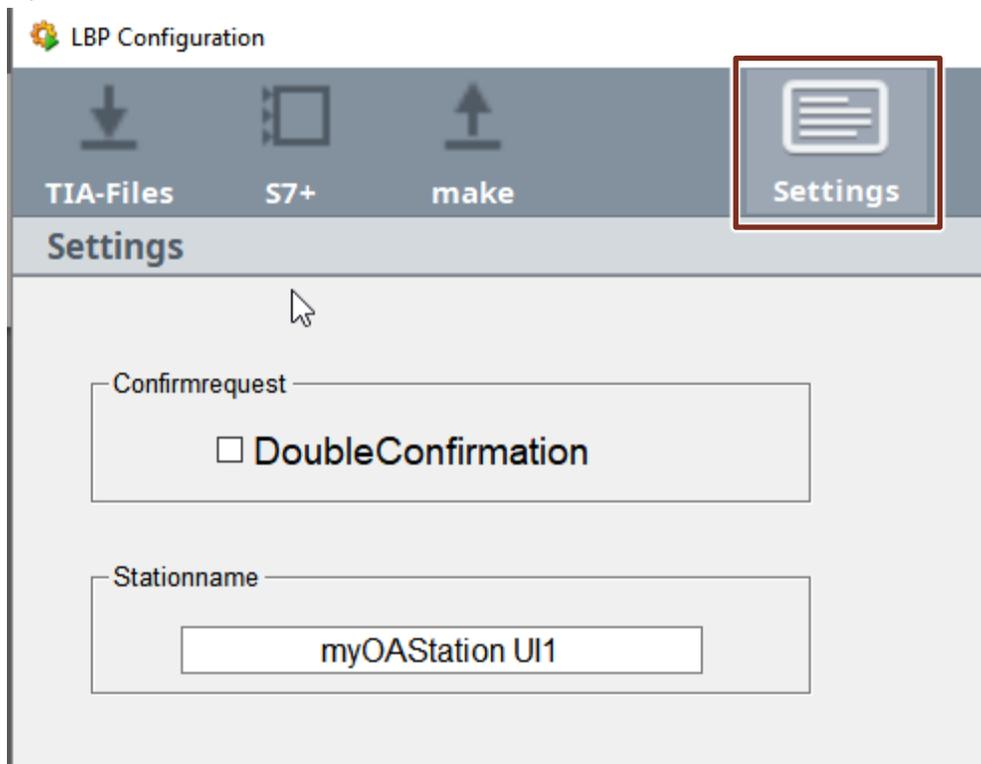
4. Set a check mark at “DoubleConfirmation” to specify whether the operating actions have to be confirmed in the running project via an additional request. Otherwise, the input may be carried out directly.
