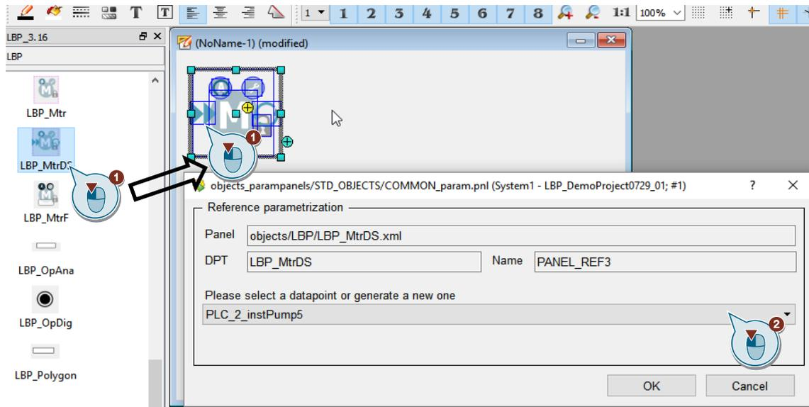
A further possibility to drag objects into the graphical surface using drag & drop is the Database Parameter Assignment Tool (PARA).
