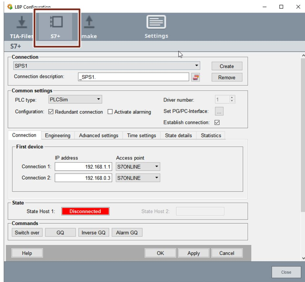
Create and name a new connection and select the desired PLC type.
