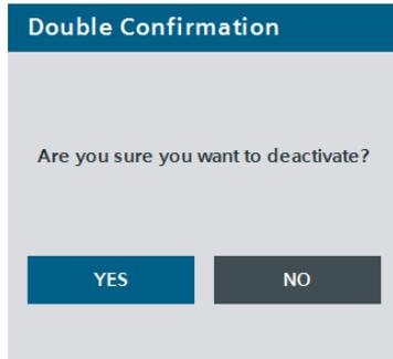
4. Create a text list with the queries for the Double Confirmation. The text is selected by the value which is passed to the script via the “cmd” interface.
