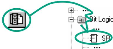
Navigate in the Program Elements catalog under **Bit Logic** until you reach the **SR** element. Double-click to insert the element.
