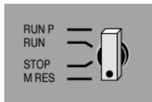
Turn the operating mode switch to the **MRES** position and hold it there for at least 3 seconds until the red "STOP" LED starts flashing slowly.
