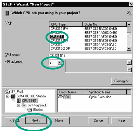
For the "Getting Started" sample project, select CPU 314. The example has been created in such a way that you can actually select the CPU you have been supplied with at any time.
