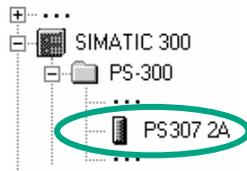
First you require a power supply module. Navigate in the catalog until you reach the **PS307 2A** and drag and drop this onto slot 1.
