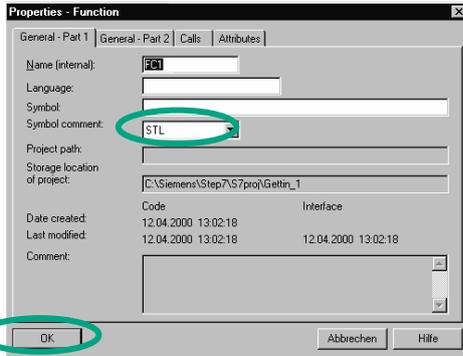
In the "Properties – Function" dialog box, accept the name FC1 and select the required programming language. Confirm the remaining default settings with **OK**.
