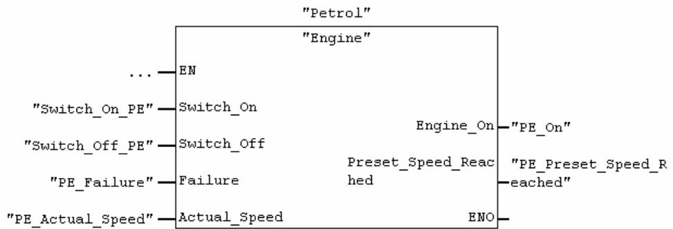
A signal "PE\_xxx" is assigned to each of the variables for the petrol engine.
