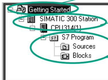
The SIMATIC station and the CPU contain the configuration and parameter data of the hardware
