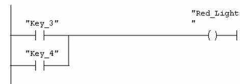
Overwrite the upper normally open contact with "Key\_3," the lower contact with "Key\_4," and the coil with "Red\_Light."
