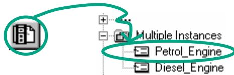
Insert the call "Petrol\_Engine" as the multiple-instance block "Petrol\_Engine" in Network 1.
