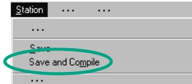
Finally, **save and compile** the distributed I/O configuration.
