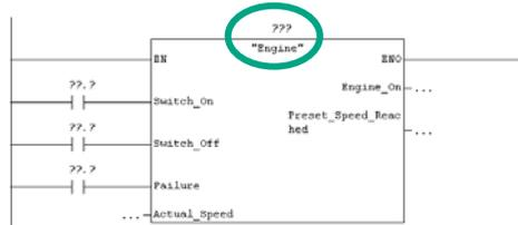
Insert a normally open contact in front of each of the following: Switch\_On, Switch\_Off, and Fault.
