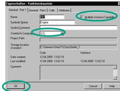
In the "Properties – Function Block" dialog box, select the language in which you want to create the block, activate the check box "**Multiple instance FB**," and confirm the remaining settings with **OK**.
