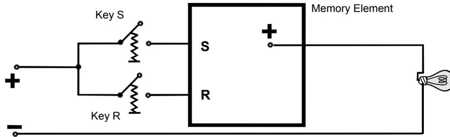
If key S is pressed, the bulb lights up and remains lit until key R is pressed.
