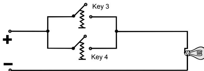
If **either** key 3 **or** key 4 is pressed, the bulb lights up.
