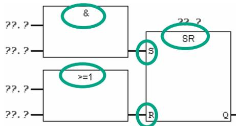
Insert an SR function in Network 1 using the Program Elements catalog (Bit Logic folder).
