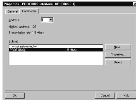
Apply the suggested address in the dialog box displayed. Select "PROFIBUS(1)" in the "Subnet" field and then apply your settings with **OK**.
