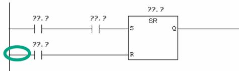
Insert another normally open contact. Select the current path immediately before this contact.
