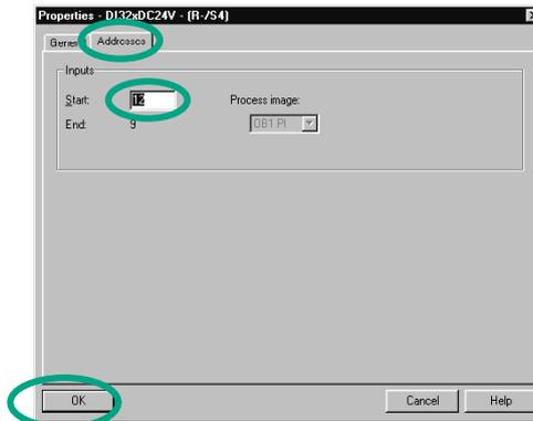
Now change the input addresses in the "Addresses" tab of the "Properties" dialog box from 6 to **12**. Close the dialog box with **OK**.
