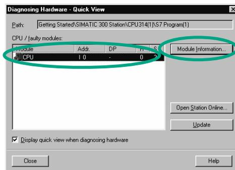
All the accessible CPUs are listed in the "Diagnosing Hardware" dialog box. The CPU with the STOP operating mode is highlighted.
