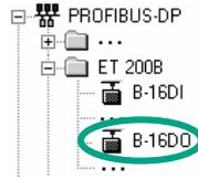
In the same way, drag and drop the module **B-16DO** onto the master system.
