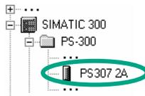
Drag and drop the power supply module **PS307 2A** into slot 1.
