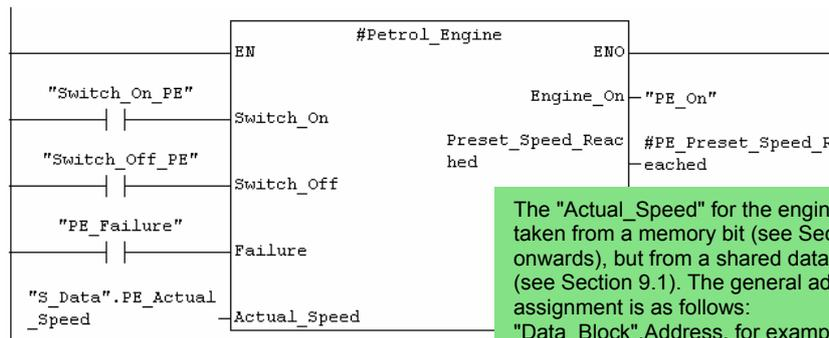
The "Actual\_Speed" for the engines is not taken from a memory bit (see Section 5.6 onwards), but from a shared data block (see Section 9.1). The general address assignment is as follows: "Data\_Block".Address, for example: "S\_Data".PE\_Actual\_Speed.
