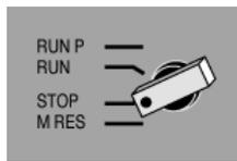
Turn the operating mode switch to the STOP position (if not already in STOP). The red "STOP" LED will light up.
