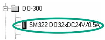
In the same way, insert the output module **SM322 DO32xDC24V/0.5A** in slot 5.
