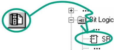
Navigate in the Program Elements catalog under **Bit Logic** until you reach the **SR** element. Double-click to insert the element.
