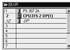
The CPU 315-2 DP already appears in the rack. If necessary, open the Hardware catalog using the menu command **View > Hardware Catalog** or the corresponding button in the toolbar.
