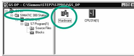
Select the folder **SIMATIC 300 Station** and double-click **Hardware**. The "HW Config" window is opened (see Section 6.1).
