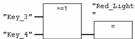
Enter "Key\_3" for the upper input, "Key\_4" for the lower input, and "Red\_Light" for the assignment.
