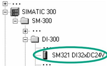
Navigate until you find the input module (DI, Digital Input) **SM321 DI32xDC24V** and insert this in slot 4. Slot 3 remains empty.
