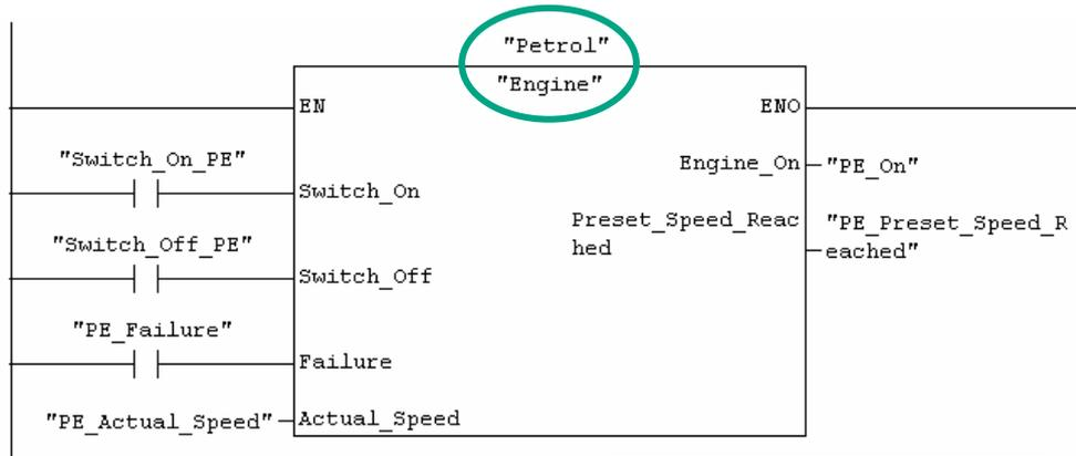
The engine-specific input and output variables (declaration "in" and "out") are displayed in the FB "Engine."
