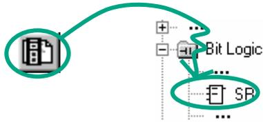
Navigate in the Program Elements catalog under **Bit Logic** until you reach the **SR** element. Double-click to insert the element.
