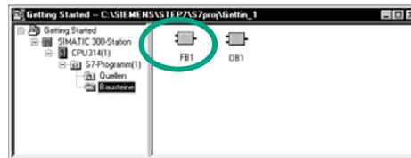
The function block **FB1** has been inserted in the Blocks folder.
