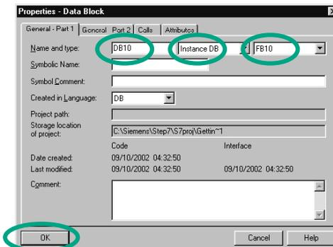
To do this, change the name of the data block to DB10 in the dialog box "Properties - Data Block", then select the application "Instance DB" in the adjacent pull-down list. In the right pull-down list, select the function block "FB10" to be assigned and confirm the remaining settings with **OK**.
