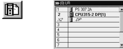
The CPU 315-2 DP already appears in the rack. If necessary, open the Hardware catalog using the menu command **View > Hardware Catalog** or the corresponding button in the toolbar.
