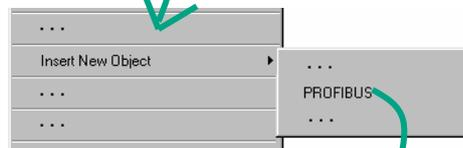
Insert the **PROFIBUS** network using the right mouse button in the right half of the window.
