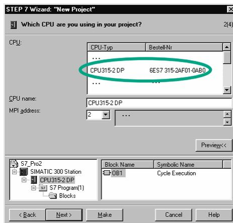
Select the **CPU 315-2DP** in the corresponding dialog box (CPU with PROFIBUS-DP network).
