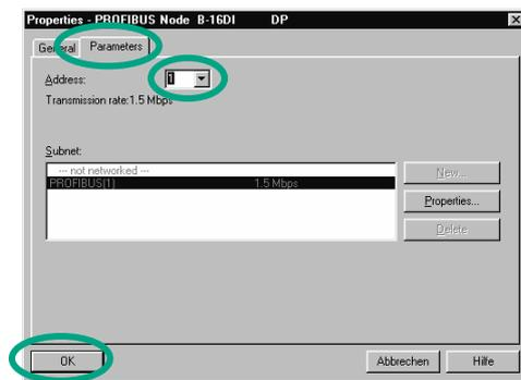
You can change the node address of the module you have inserted in the "Parameters" tab of the "Properties" dialog box. Confirm the suggested address with **OK**.
