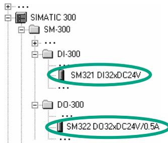
In the same way, insert the I/O modules **DI32xDC24V** and **DO32xDC24V/0.5A** in slots 4 and 5.
