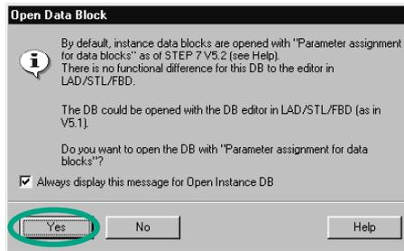
Confirm the subsequent dialog with **Yes** to assign parameters to the instance data blocks.
