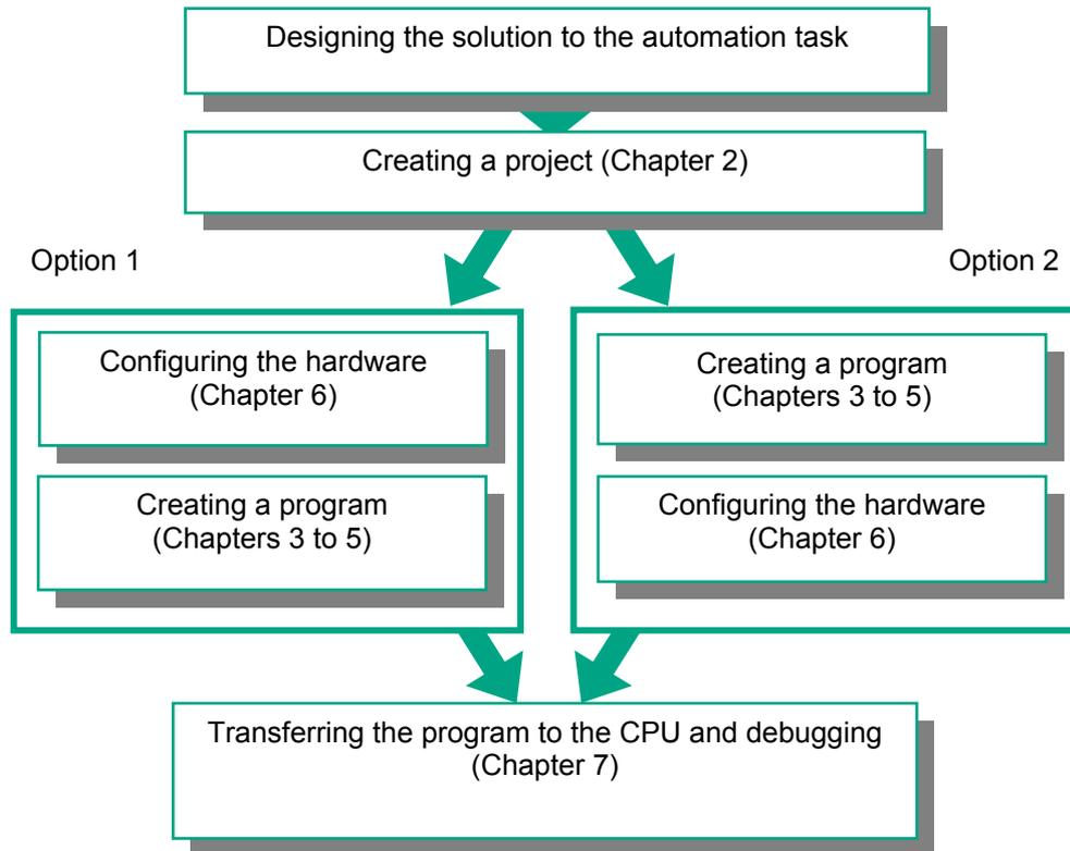
If you are creating comprehensive programs with many inputs and outputs, we recommend you configure the hardware first. The advantage of this is that STEP 7 displays the possible addresses in the Hardware Configuration Editor.
