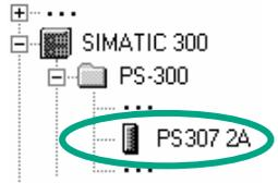
First you require a power supply module. Navigate in the catalog until you reach the **PS307 2A** and drag and drop this onto slot 1.
