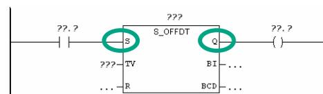
Insert a normally open contact in front of input **S**.
