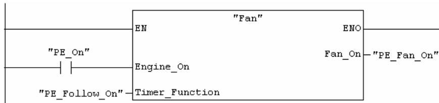
Program the call for the function FC1 in Network 7 using the addresses for the diesel engine. You can do this in the same way as for the previous network (you have already added the addresses for the diesel engine to the symbol table).
