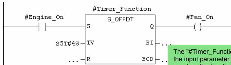
The "#Timer\_Function" is started with the input parameter "#Engine\_On." Later on when the function is called in OB1, it will be supplied once with the parameters for the petrol engine and once with the parameters for the diesel engine (for example, T1 for "PE\_Follow\_on"). You will enter the symbolic names of these parameters later in the symbol table.
