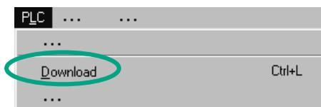
Select the **Blocks** folder in the offline window and then download the program to the CPU using the menu command **PLC > Download**. Confirm the prompt with **OK**.
