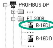
Navigate in the Hardware catalog until you reach the module **B-16DI** and insert this module in the master system (drag the object to the master system until the cursor changes to a "+" sign; then drop the object).
