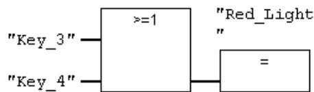
Enter "Key\_3" for the upper input, "Key\_4" for the lower input, and "Red\_Light" for the assignment.
