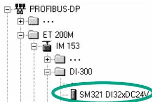
The ET200M itself can have additional I/O modules. Select, for example, the module **DI32xDC24V** for slot 4 and double-click this module to insert it.
