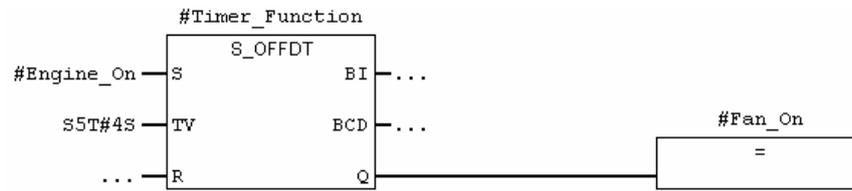
In order for the timer function to be processed, you need to call the function in a block which is higher up in the block hierarchy (in our example, in OB1).
