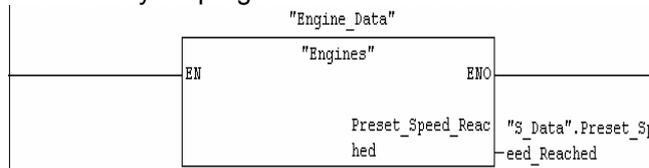
The output signal "Setpoint\_Reached" for FB10 ("Engines") is passed on to the variable in the shared data block.
