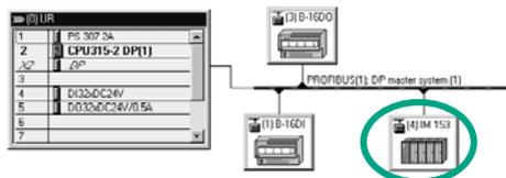
Select the **ET200M** in the network. The free slots for the ET200M are displayed in the lower configuration table.
