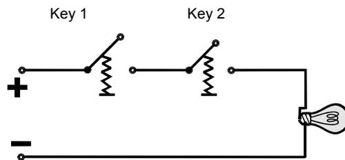
If both Key 1 **and** Key 2 are pressed, the bulb lights up.
