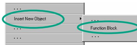
The pop-up menu for the right mouse button contains the most important commands from the menu bar. Insert a **function block** as a new object.
