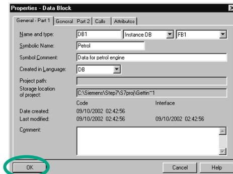
Apply the name DB1 in the "Properties Data Block" dialog box, then select the application "Instance DB" in the adjacent pull-down list and apply the name of the function block "FB1" assigned. Apply all the settings displayed in the "Properties" dialog box with **OK**.
