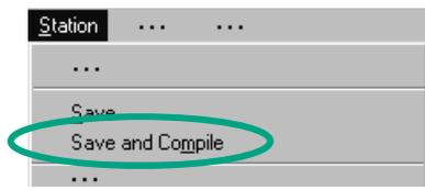
The data are prepared for transfer to the CPU using the menu command **Save and Compile**.
