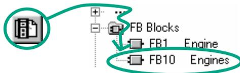
Insert a new network at the end of OB1 and add the call for **FB10** ("Engines").
