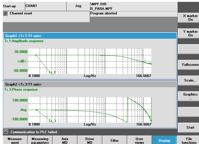
Figure 8-7 Optimized position control loop
