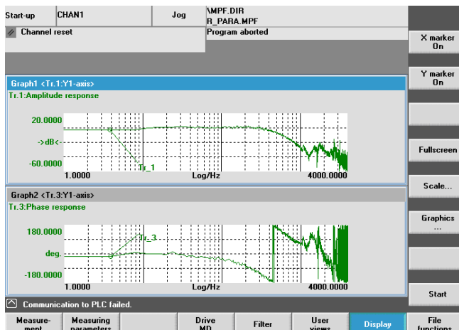
Figure 8-6 Optimized speed control loop
