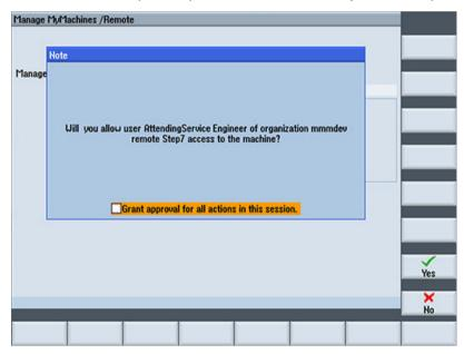
3. If the machine operator presses the "No" softkey, access is denied for the remote user. The remote user receives the following message:
