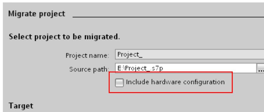
The first step after migrating without hardware configuration is to change the unspecified CPU to a specified CPU.
