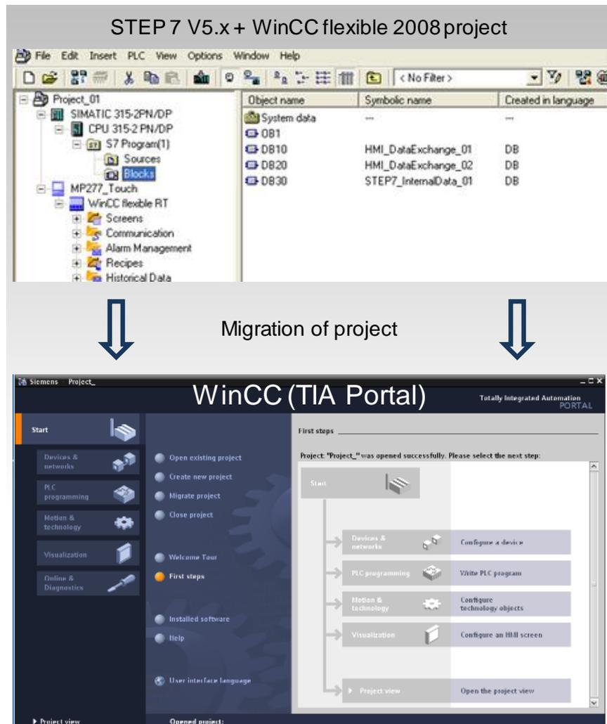
The application example essentially shows the prerequisites that are necessary for the upgrade/migration of an HMI operator panel.
