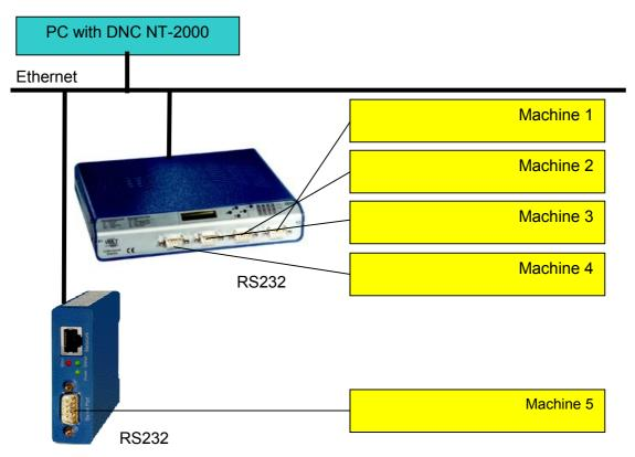
Currently Siemens does not offer these interface converters. We are e.g. using:
