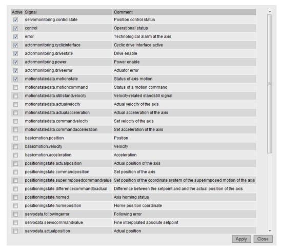
Figure 4-15 **Extended...** button: Selection of variables
