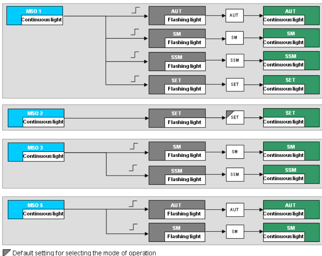
Fig. 6-22: Diagram of TRANSLINE Modes of Safe Operations
