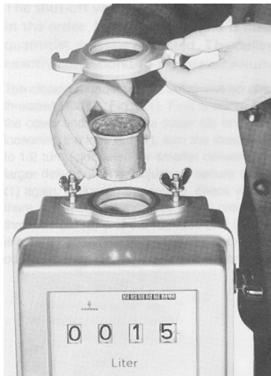
Fig. 3/1 Replacing the drying cartridge
