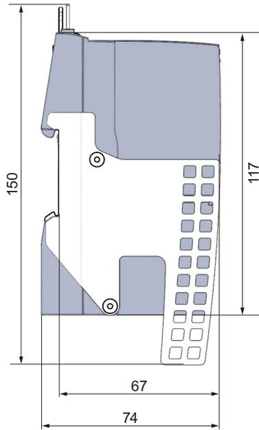
Figure 15-2 Dimension drawing CPU 1515SP PC2, side view
