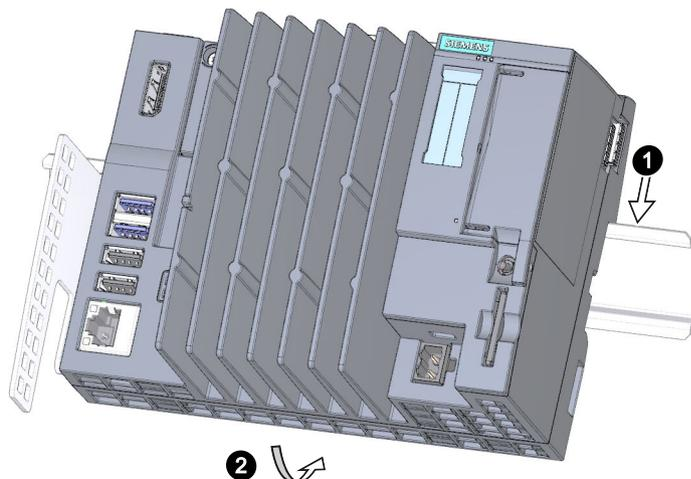
Figure 7-1 Installing the CPU 1515SP PC2
