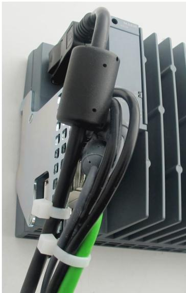
Figure 8-3 Secured cables
