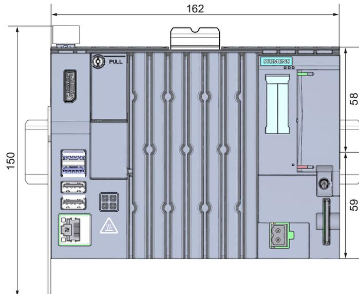
Figure 15-1 Dimension drawing CPU 1515SP PC2, front view
