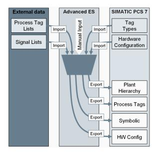
This results in Simatic PCS 7 creating the technological hierarchy, control module instances with signal and parameter settings, as well as the hardware configuration.
