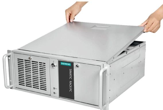
3. Lift the cover from the back and remove it.
