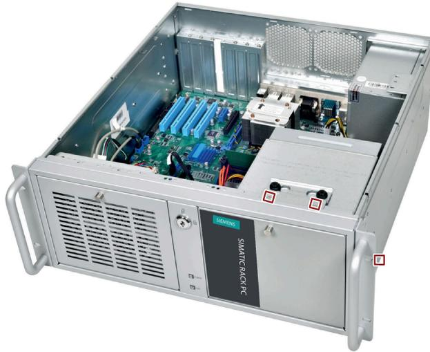
5. Lift the drive cage completely out of the device.
