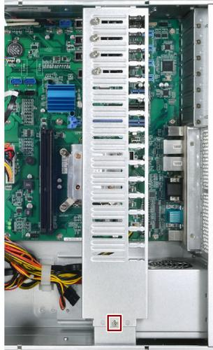
2. Remove the slot bracket of the slot for the expansion card.
