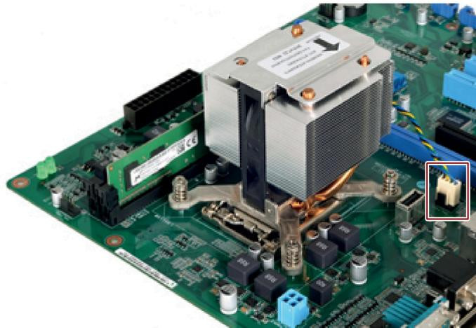
3. Remove the highlighted screws.
