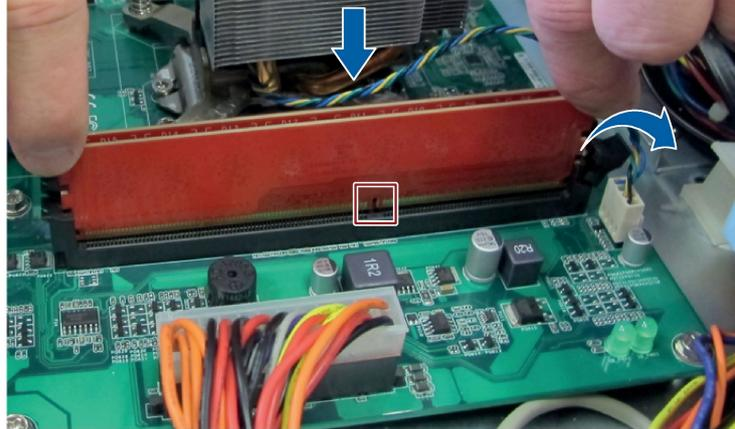
3. Insert and press the memory module into the socket until the retaining clips snap back to the original place, and the Memory Module is seated properly.
