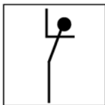
Figure 2-2 Symbol for mirror contacts in a switching device
