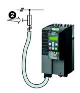
After the power supply has been switched on, the inverter copies its changed settings to the memory card.
