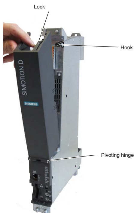
Figure 3-4 Opening the front cover using the D4x5-2 as an example
