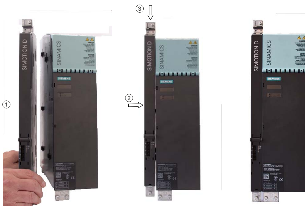
Figure 2-8 Steps in mounting the CX32-2 on a booksize line module
