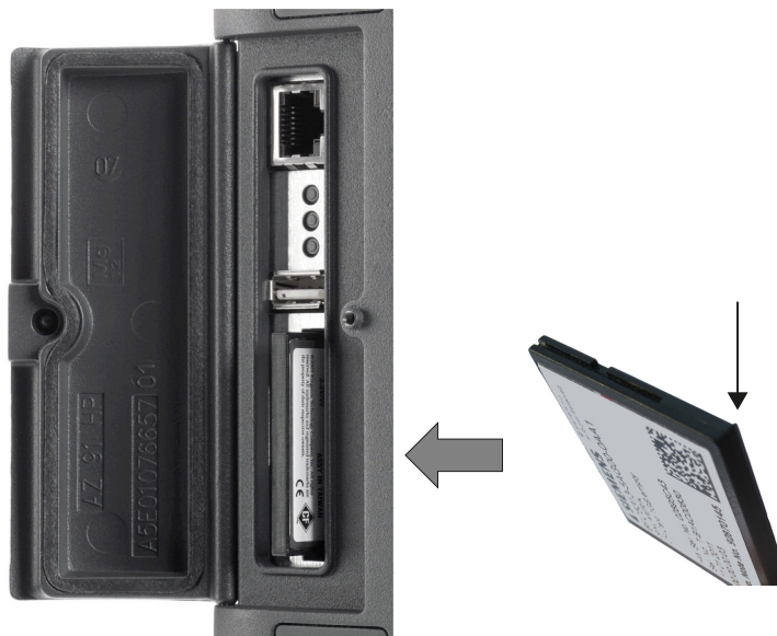
Figure 2-8 Direction to insert the user CompactFlash card
