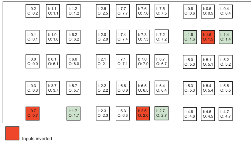
Figure 7-26 Inputs and outputs of the MCP 310C PN keyboard
