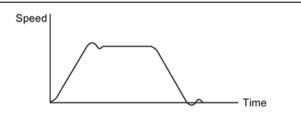
**Example 2**: The function of PI/P switching can be used to suppress overshooting and undershooting when speed loop gain is increased
