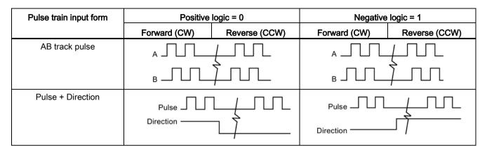
For both forms, positive logic and negative logic are supported.
