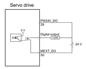
The digital outputs 4 to 6 support the wiring of both the NPN and the PNP types as illustrated below:
