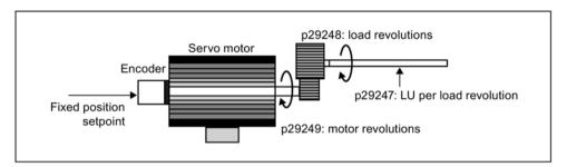
The unit of the fixed position setpoint is the Length Unit (LU). All subsequent position setpoint, related speed value, and acceleration value will maintain the LU as the unit in internal position control mode.
