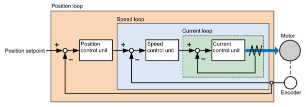
In theory, frequency width of the inside control loop **must** be wider than that of the outer control loop; otherwise, the whole control system can vibrate or have a low response level. The relationship between the frequency widths of these three control loops is as follows:
