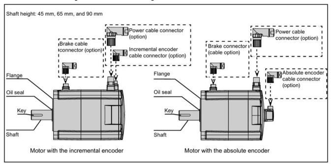
High inertia motors with angular connectors
