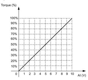
In this case, analog input of 5 V corresponds to 50% of rated torque and 10 V corresponds to 100% of rated torque.
