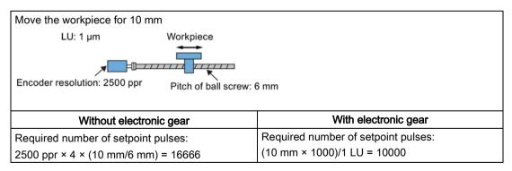
The electronic gear ratio is a multiplier factor to pulse train setpoint. It is realized with a numerator and a denominator. Four numerators (p29012[0], p29012[1], p29012[2]. p29012[3]) and one denominator (p29013) are used for the four electronic gear ratios.
