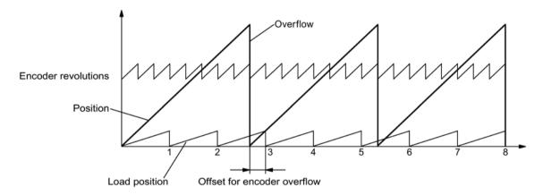
For each encoder overflow, there is a load-side offset of 1/3 load revolution, after three encoder overflows, the motor and load zero position coincide again. The position of the load can no longer be clearly reproduced after one overflow.
