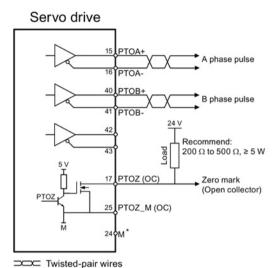
\* Connected to the reference ground of the host controller
