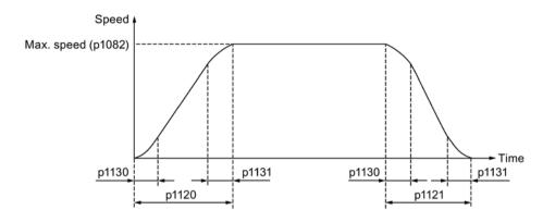
You can see the properties of the S-curve ramp-function generator from the diagram below:
