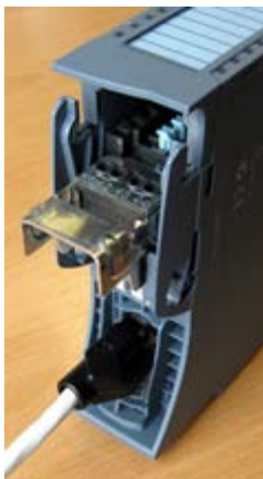
Image 4-8 Ethernet cable connected to module
