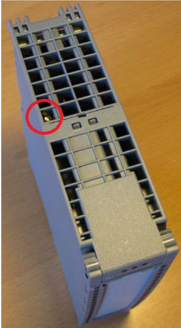
Image 5-1 Switch position in the enclosure
