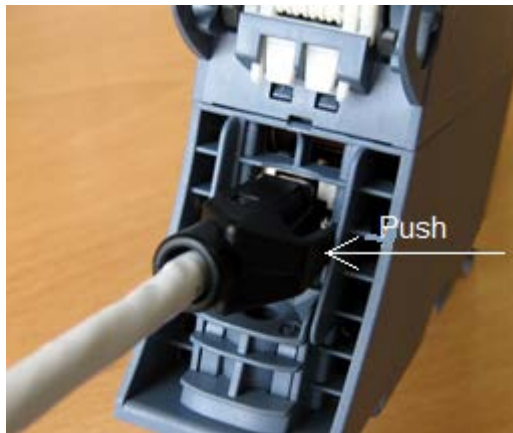
Image 4-9 Press the Ethernet cable into the socket
