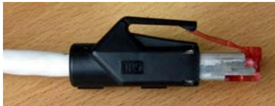
Image 4-10 Ethernet plug with release lever
