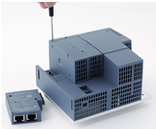
Figure 4-11 Installation of the modules
