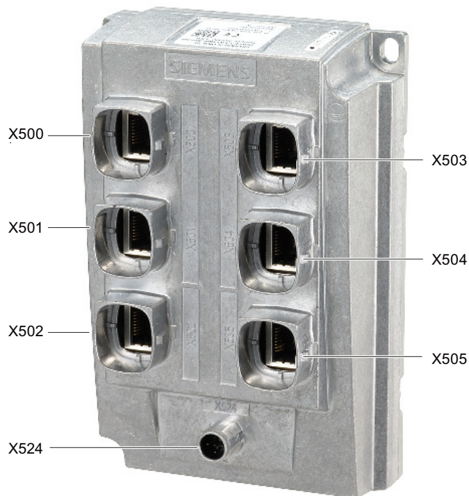
X500 ... X505 DRIVE-CLiQ interfaces X524 Electronics power supply Figure 5-68 DME20 connections
