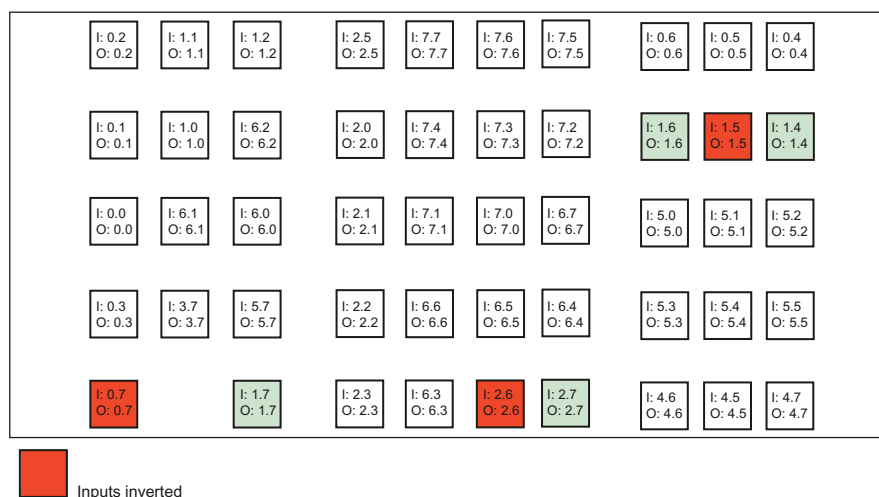
Figure 7-26 Inputs and outputs of the MCP 310C PN keyboard
