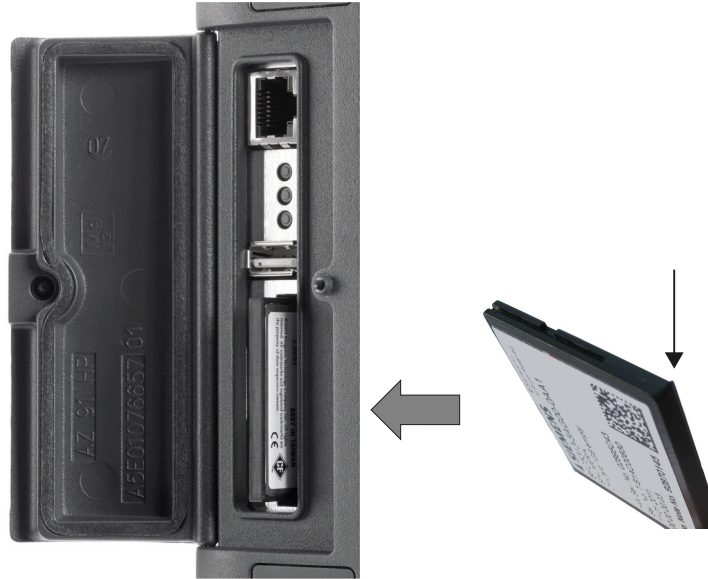
Figure 2-8 Direction to insert the user CompactFlash card
