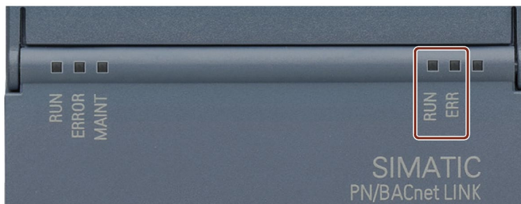
Figure 10-2 Status LEDs BACnet bus
