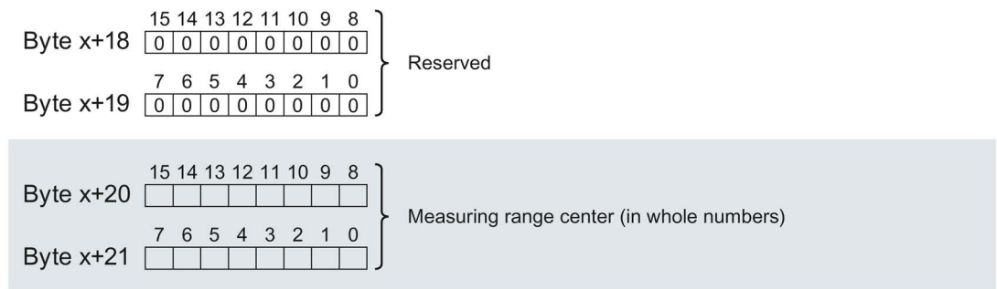
Figure A-3 Structure of byte x to x+21 for channel 0 to 3 - S7 representation
