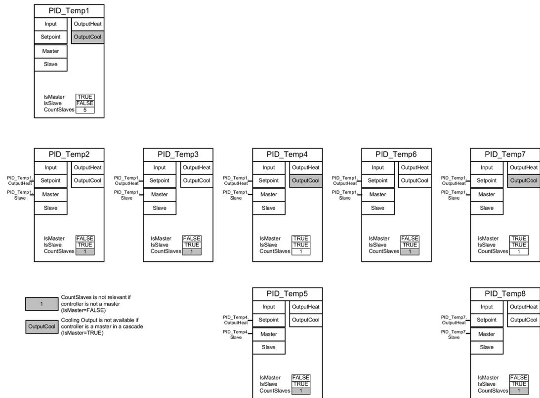
Figura 10-8 PID\_Temp\_Cascading\_communication\_connection
