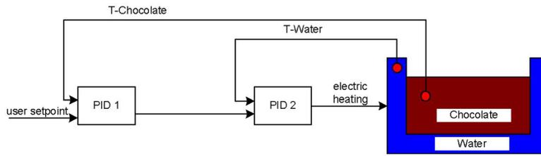
Figura 10-7 PID\_Temp\_Cascade\_Operation\_Block\_Diagram
