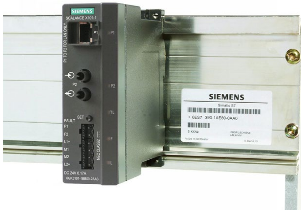
Figure 4-3 Standard rail mounting X-100MC
