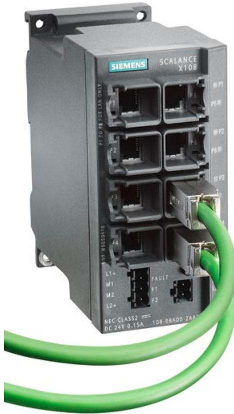
Figure 5-2 Plugging in the IE FC RJ45 Plug 180
