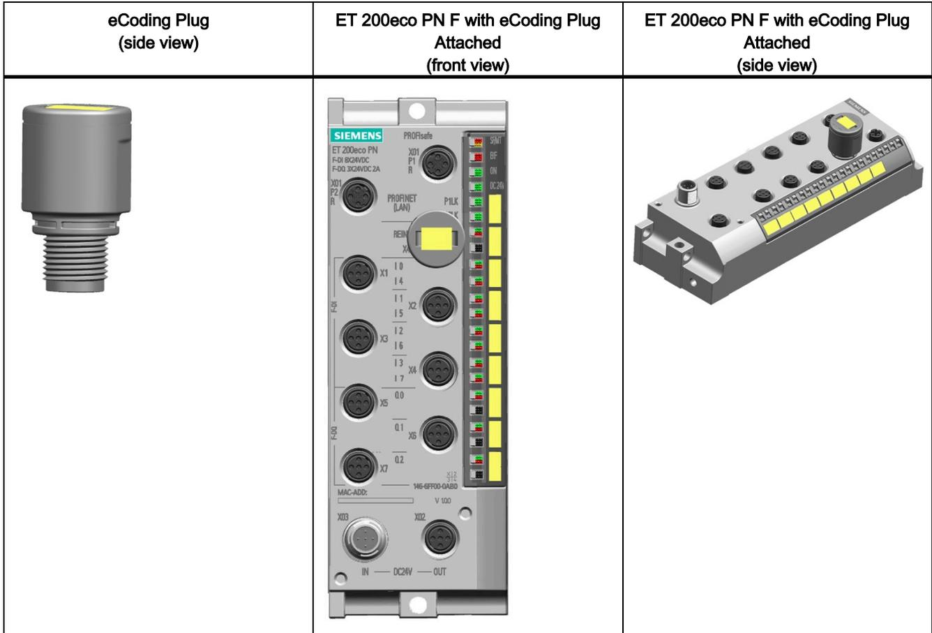
The eCoding plug stores the PROFIsafe source address, the PROFIsafe destination address, and a CRC external to the module. The eCoding plug occupies the X40 M12 connector, utilizing a B-coded plug. You use the eCoding plug to facilitate module replacement.
