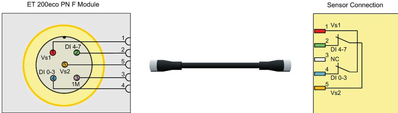
Note: To incorporate F-DI Application Mode 3 into a SIL 3-rated application, the sensor must be an appropriately qualified device.
