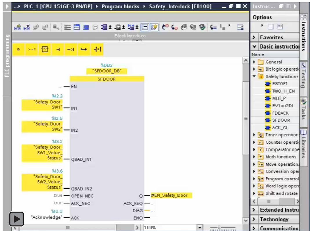
1. In the interface of the "Safety\_Interlock" F-BB, create a static tag of data type "Bool" named "EN\_Safety\_Door" (Enable safety door).
