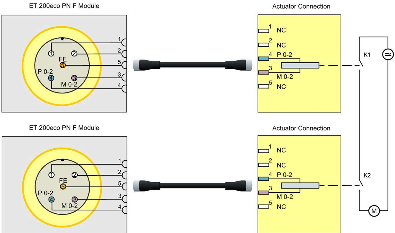
Note: The Application Mode 4 configuration achieves SIL 3/Category 4/PL e if the CPU checks the relay status (feedback) using a separate digital input.
