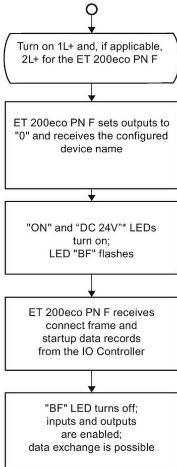
\* "DC 24V" only for digital output and if 2L+ is connected
