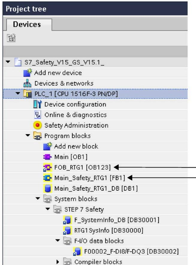
The first step in programming of the safety program is the main safety block. The program calls the main safety block (which is an F-FB (with instance DB)) from the "Fail-Safe Organization Block" (F-OB) (cyclic interrupt OB), assigned in each F-runtime group. By default, the F-OB has a higher priority than other standard OBs.
