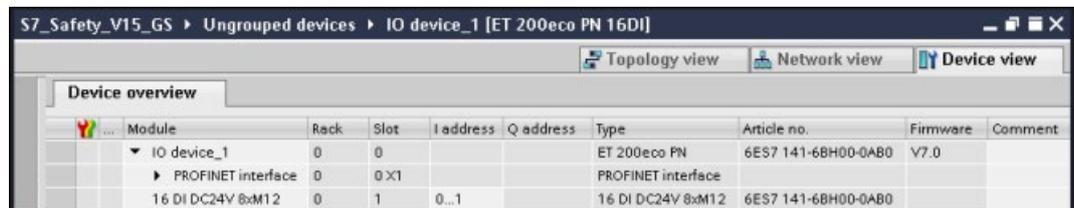
2. Return to the "Device view" and select the ET 200eco PN 16DI. Under the "Properties" tab, select the "IO tags" tab. Here, you can define tags for each channel:
