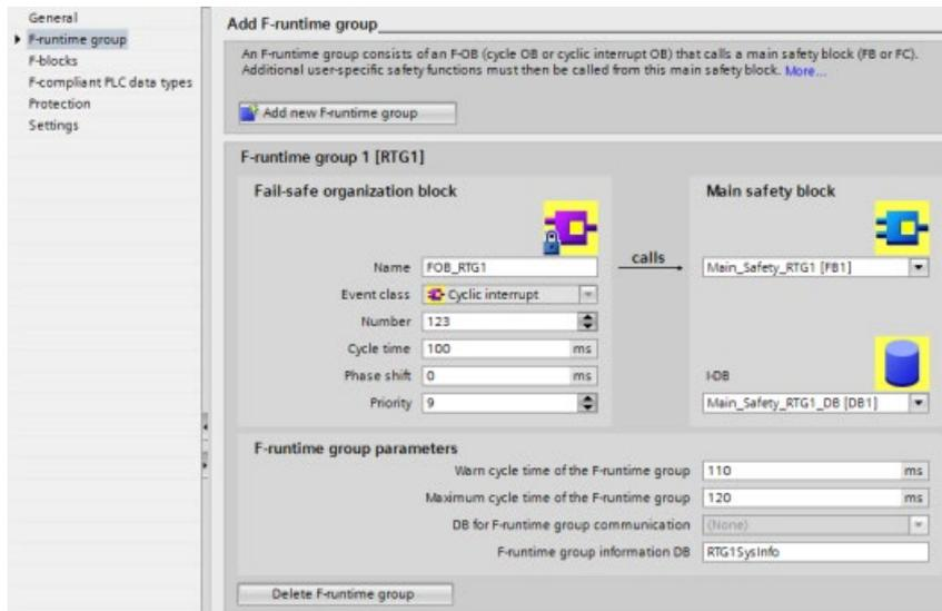
The cyclic interrupt OB (FOB\_RTG1 [OB123]) calls the main safety block (Main\_Safety\_RTG1 [FB1]) by default. The program calls the F-blocks that you create from the main safety block. You can change the calling block and the called block at any time.
