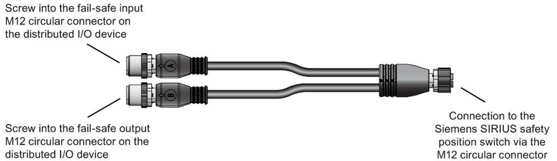
The wiring of the inverted Y cable is shown below:
