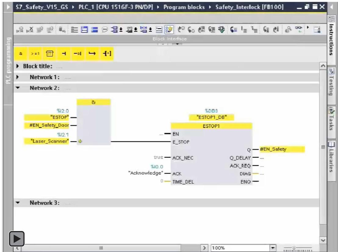
1. In the interface of the "Safety\_Interlock" F-FB, create a static tag of data type "Bool" named "EN\_Safety" (Enable safety circuit).
