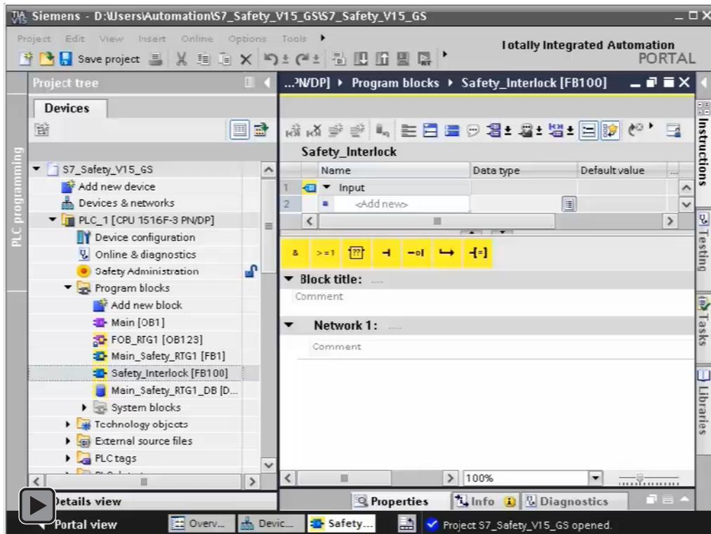
1. Insert an F-FB. Go to the "Program blocks" folder of the fail-safe CPU and double-click "Add new block".
