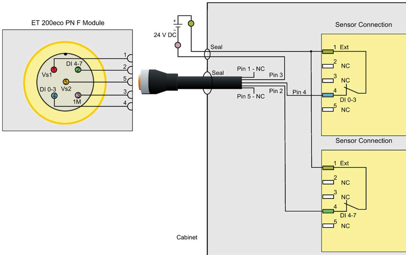
Note: To incorporate F-DI Application Mode 2 into a SIL 2-rated application, the sensor must be an appropriately qualified device.
