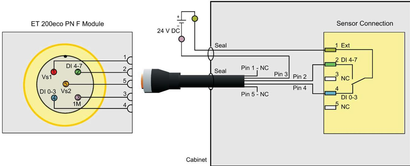
Note: To incorporate F-DI Application Mode 6 into a SIL 3-rated application, the sensor must be an appropriately qualified device.
