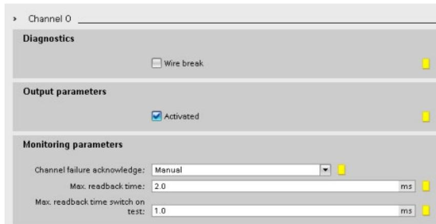
2. Disable the unused DQ channels 1 and 2 by clearing the "Activated" check box.
