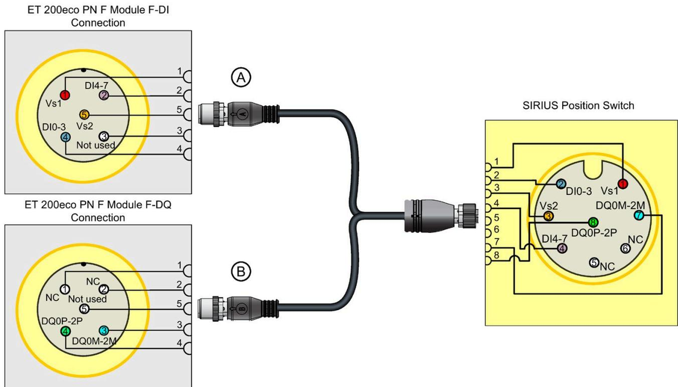
Note: To incorporate F-DI/F-DQ Application Mode 1 into a SIL 3-rated application, the sensors must be appropriately qualified devices: Either SIL 3 or SIL 2 with the Systematic Capability rules defined in the SIRIUS documentation. For further information, refer to the Industrial Controls, Detecting devices SIRIUS 3SE5/3SF1/3SE66/3SE67 position switches Configuration Manual (<https://support.industry.siemens.com/cs/us/en/view/43920150>).
