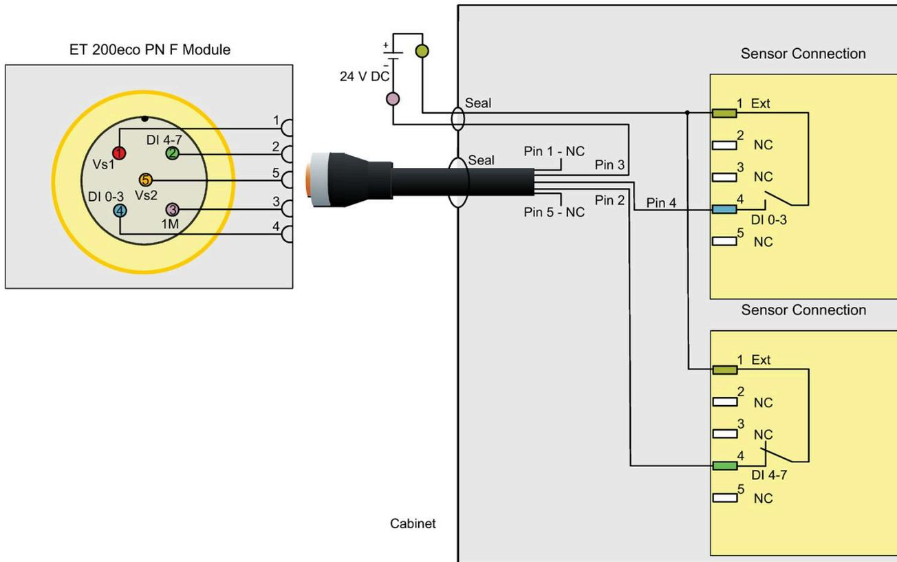
Note: To incorporate F-DI Application Mode 8 into a SIL 3-rated application, the sensors must be appropriately qualified devices: Either SIL 3 or SIL 2 with Systematic Capability rules defined in IEC 61508-2:2010 observed (sufficient independence in design and application or SC3).
