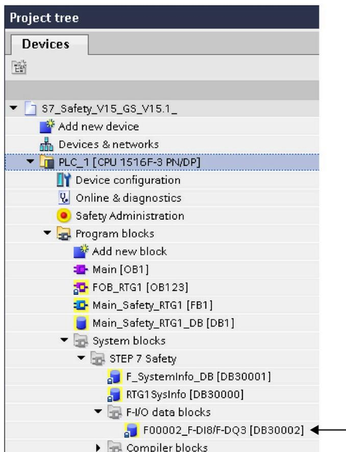
The default name of the F-I/O DB is formed from the fixed prefix "F", the start input address of the fail-safe module, and the names entered in the properties for the fail-safe module in the hardware and network editor.
