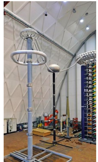
UHV arrester prepared for testing in the HV test laboratory
