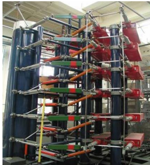
Test generator supplying both impulse voltages (1.2/50 \mu s and 250/250 \mu s) and impulse currents (8/20 \mu s and 30/60 \mu s)
