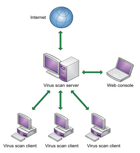
Depending on the manufacturer it may also be possible to use multiple virus scan servers which can be arranged in parallel or in a hierarchy.
