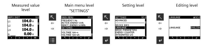
Depending on the device version and firmware status, the availability of the measured values may vary in the measured value and main menu levels. The parameter selection options at the setting and editing levels also depend on the device version and firmware status.
