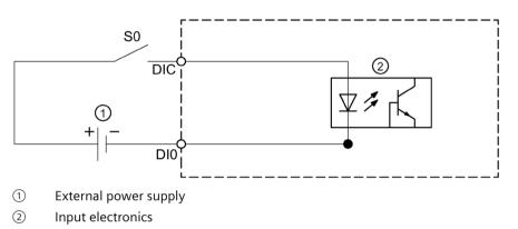
Figure 2-1 Block diagram: Digital input
