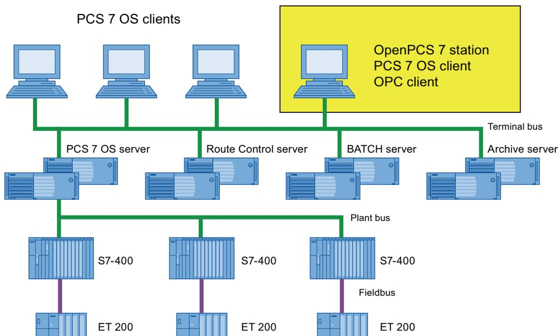
The OPC client can also run on a separate computer. This configuration is intended for small to medium-sized plants.
