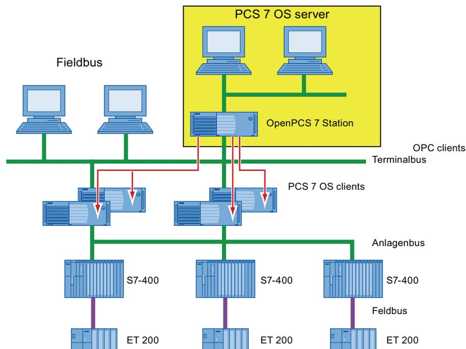
Depending on the system configuration, the OpenPCS 7 station can provide data from various OS servers and from the central archive server. The OpenPCS 7 station hides the distribution of the data in terms of:
