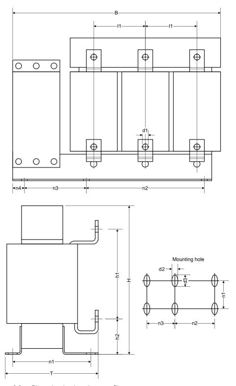
Figure 6-2 Dimension drawing, sine-wave filter
