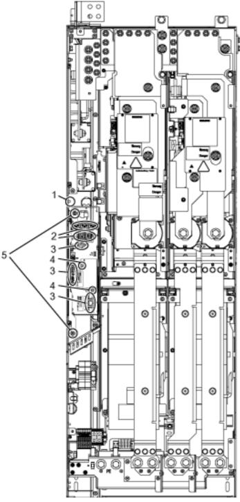
Figure 8-15 Replacing the Control Interface Module, Motor Module, frame size HX
