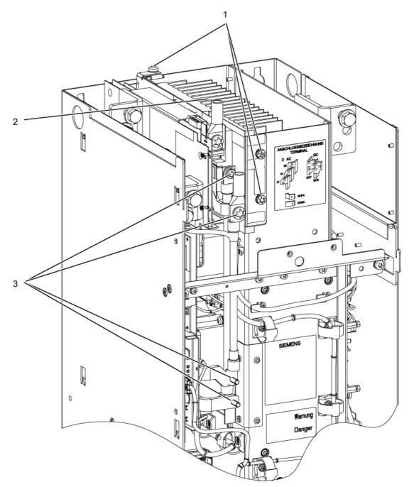
Figure 5-12 Installing the Braking Module in a Basic Line Module, frame size FB
