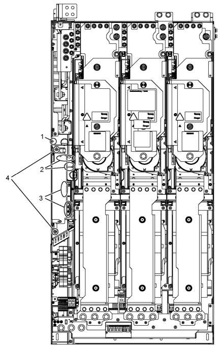
Figure 8-18 Replacing the Control Interface Board, Smart Line Module, Active Line Module, and Motor Module, frame size JX
