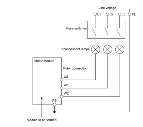
Figure 8-32 Forming circuit for Motor Modules
