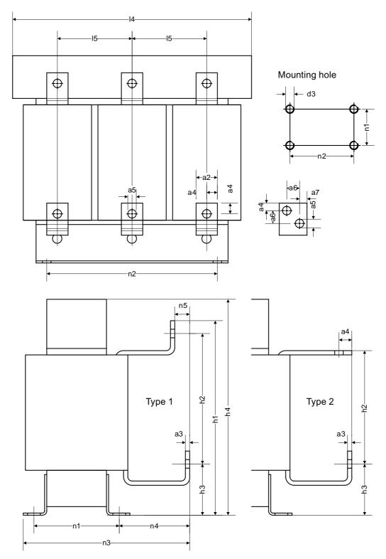
Figure 6-3 Dimension drawing, motor reactor
