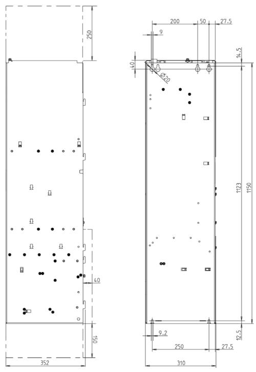
Figure 3-4 Dimension drawing, Basic Line Module, frame sizes FB, side view, front view
