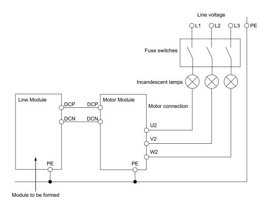
Figure 8-31 Forming circuit for Line Modules
