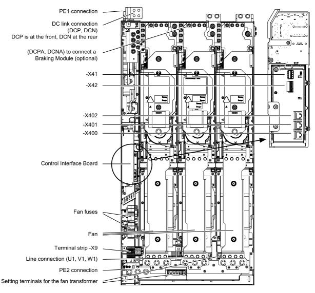
Figure 3-25 Active Line Module, frame size JX
