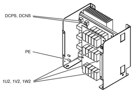
Figure 6-4 Interface overview, voltage peak limiter, type 1
