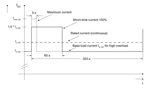
Figure 3-32 High overload
