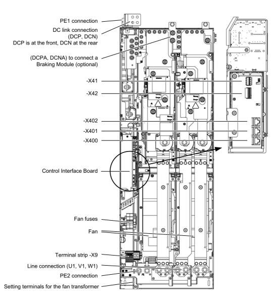
Figure 3-24 Active Line Module, frame size HX
