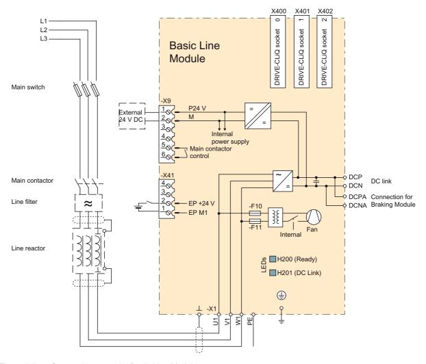
Figure 3-3 Connection example: Basic Line Module
