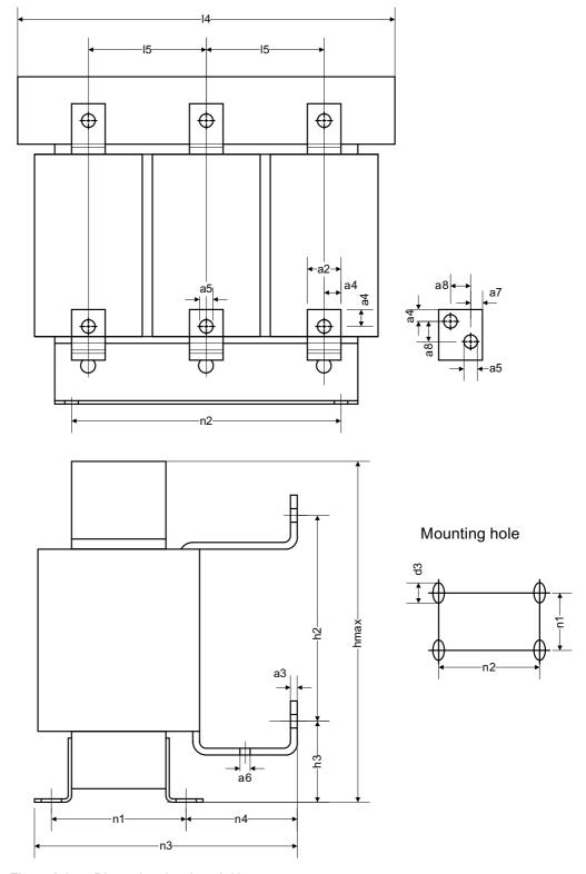
Figure 6-9 Dimension drawing, dv/dt reactor
