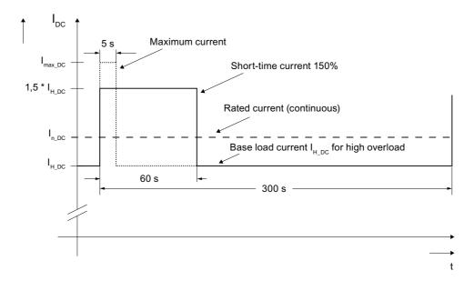
Figure 3-19 High overload
