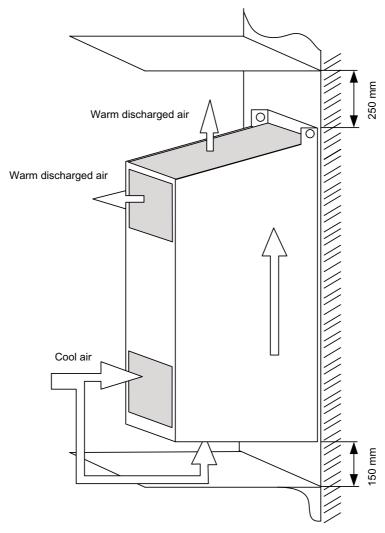
Figure 7-3 Air guidance for Smart Line Module, Active Line Module, Motor Module, frame sizes FX, GX
