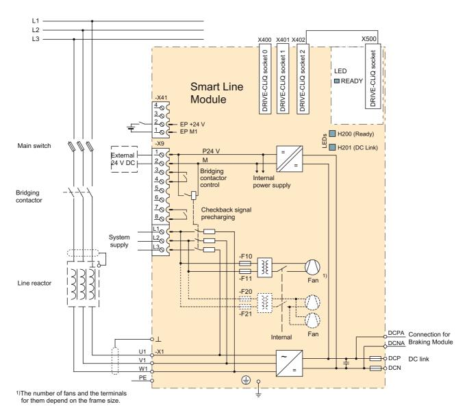
Figure 3-13 Smart Line Module wiring diagram
