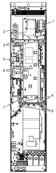
Figure 8-5 Replacing the power block, Smart Line Module, Active Line Module, and Motor Module, frame size GX
