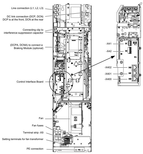
Figure 3-1 Basic Line Module, frame size FB
