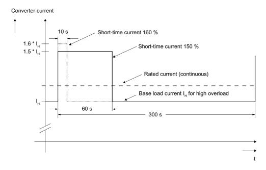
Figure 4-17 High overload
