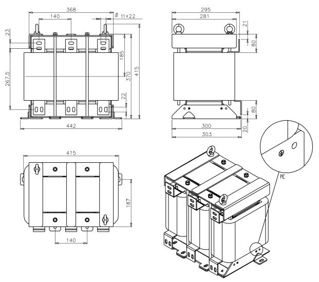
Figure 2-7 Dimension drawing of line reactor 6SL3000-0EE37-6AA0, all dimensions in mm
