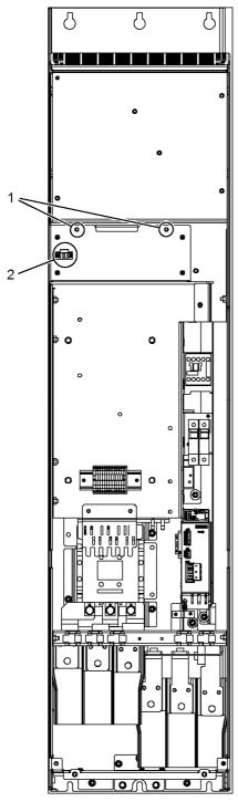
Figure 8-25 Replacing the fan, Active Interface Module, frame size FI
