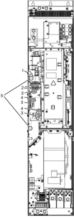
Figure 8-13 Replacing the Control Interface Module, Motor Module, frame size GX
