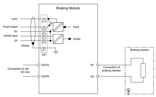
Figure 5-5 Connection example for Braking Module
