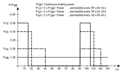
Figure 5-16 Duty cycle for braking resistors
