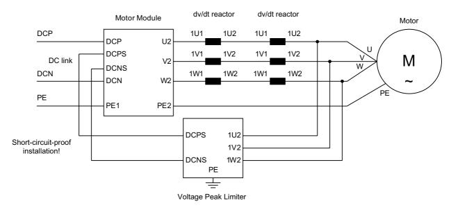
Figure 6-8 Connecting a dv/dt filter plus Voltage Peak Limiter for versions with two dv/dt reactors
