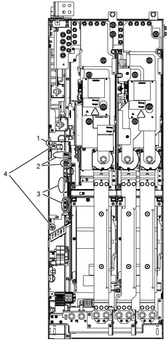
Figure 8-16 Replacing the Control Interface Board, Smart Line Module, Active Line Module, and Motor Module, frame size HX
